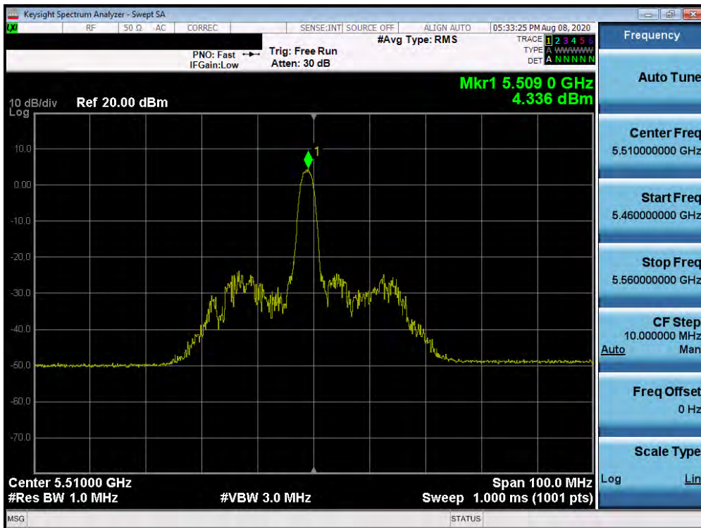
Plot 7-124. Power Spectral Density Plot SISO ANT1 (40MHz BW 802.11ax – 26 Tones (UNII Band 2C) – Ch. 102)
