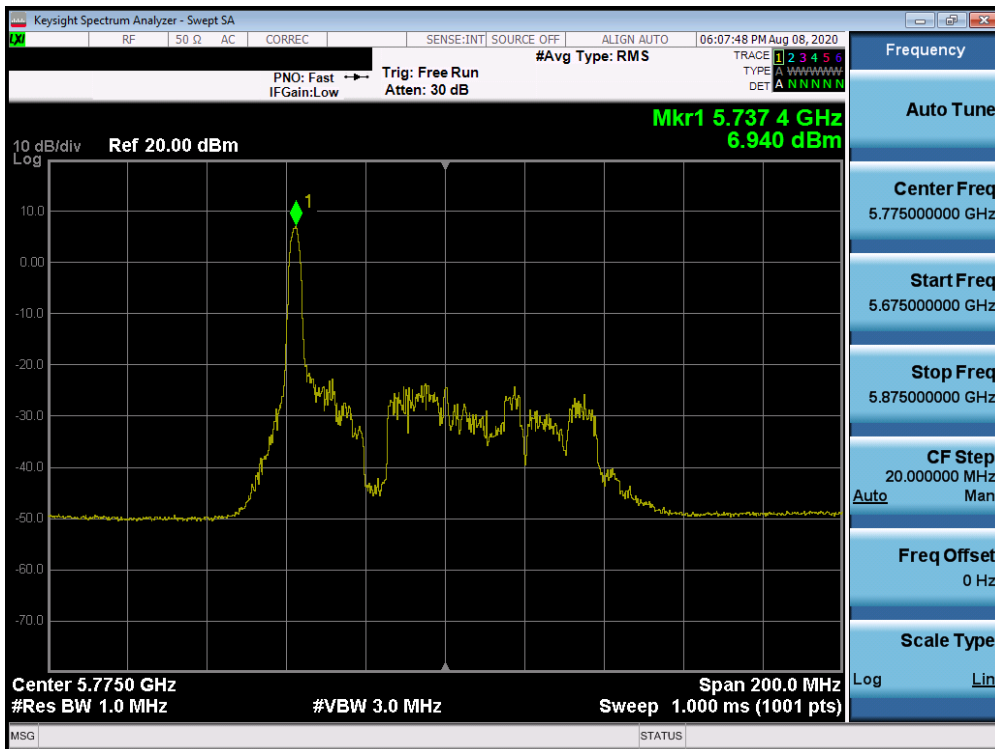
Plot 7-189. Power Spectral Density Plot SISO ANT2 (80MHz BW 802.11ax – 26 Tones (UNII Band 3) – Ch. 155)
