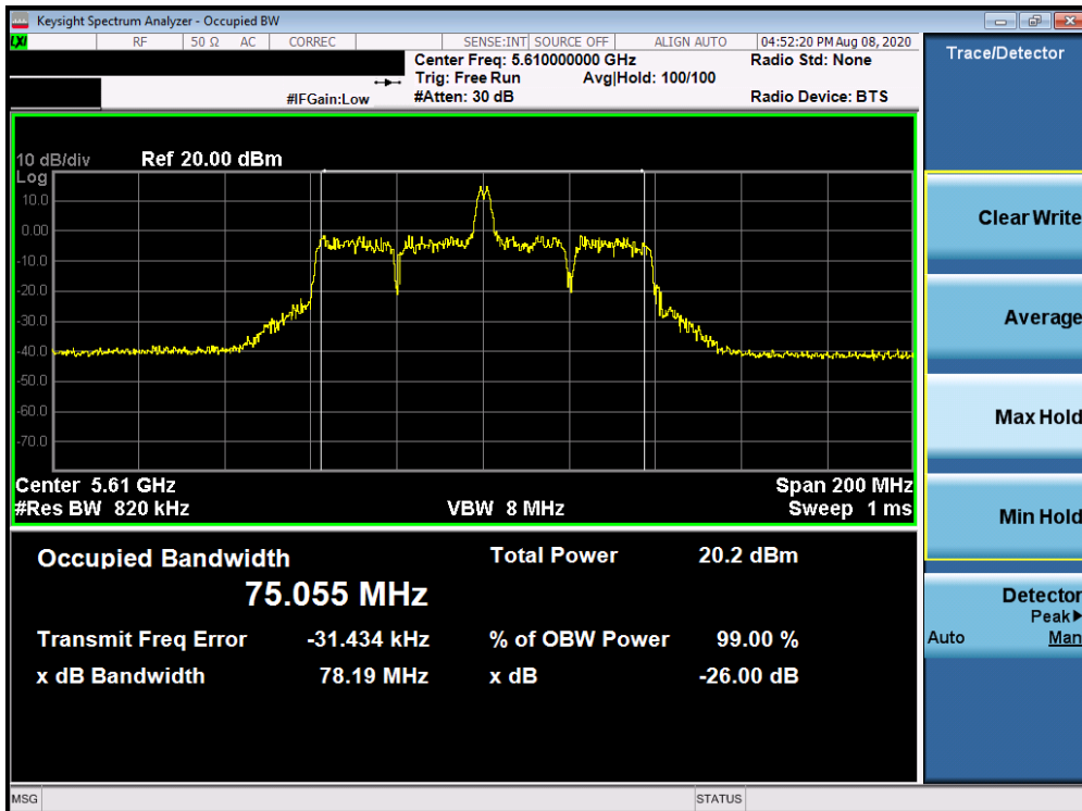
Plot 7-62. 26dB Bandwidth Plot SISO ANT2 (80MHz BW 802.11ax – 26 Tones (UNII Band 2C) – Ch. 122)
