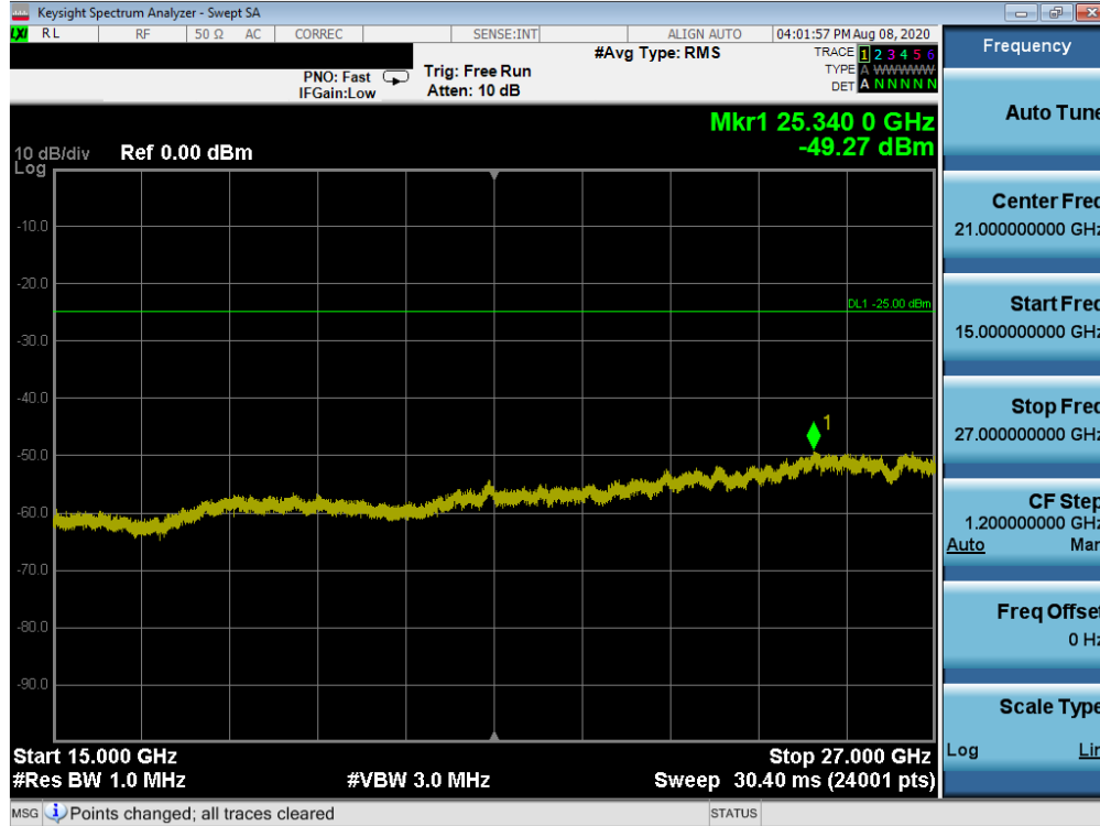
Plot 7-33. Conducted Spurious Plot (LTE Band 7 - 20MHz QPSK - RB Size 1, RB Offset 0 - High Channel)
