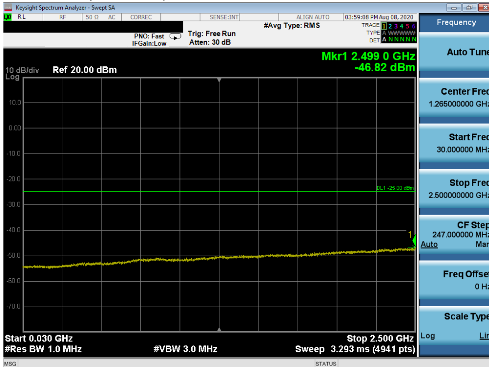
Plot 7-28. Conducted Spurious Plot (LTE Band 7 - 20MHz QPSK - RB Size 1, RB Offset 0 - Mid Channel)
