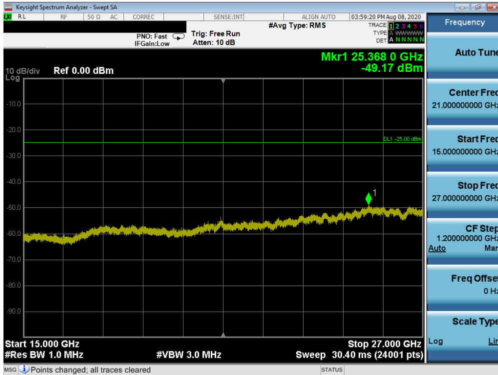
Plot 7-30. Conducted Spurious Plot (LTE Band 7 - 20MHz QPSK - RB Size 1, RB Offset 0 - Mid Channel)
