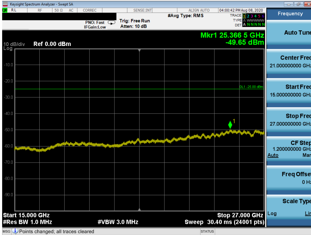
Plot 7-27. Conducted Spurious Plot (LTE Band 7 - 20MHz QPSK - RB Size 1, RB Offset 0 - Low Channel)
