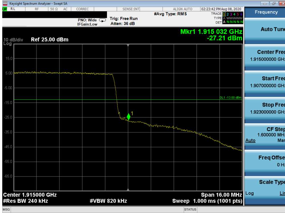
Plot 7-60. Upper Band Edge Plot (LTE Band 25 - 20MHz QPSK – Full RB Configuration)
