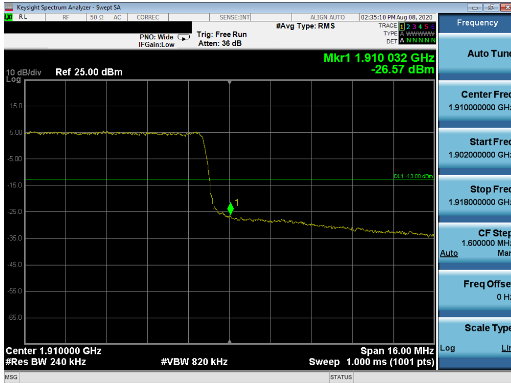
Plot 7-58. Upper Band Edge Plot (LTE Band 2 - 20MHz QPSK – Full RB Configuration)
