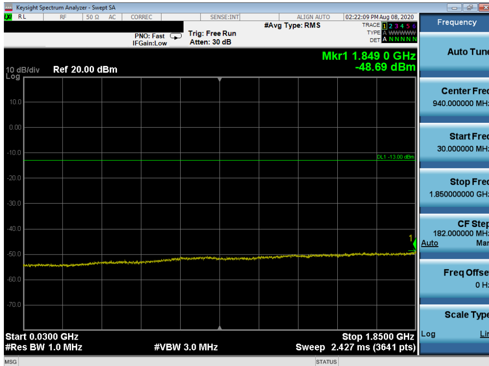
Plot 7-41. Conducted Spurious Plot (LTE Band 25/2 - 20MHz QPSK - RB Size 1, RB Offset 0 - Mid Channel)
