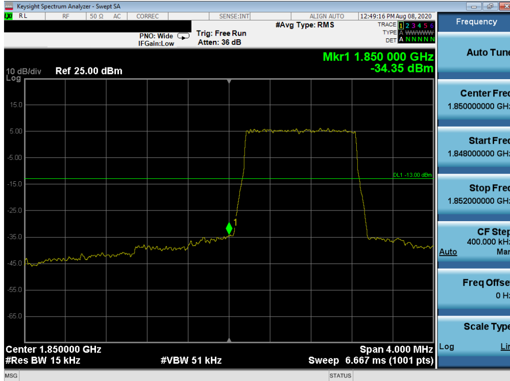
Plot 7-86. Lower Band Edge Plot (LTE Band 25/2 – 1.4MHz QPSK – Full RB Configuration)
