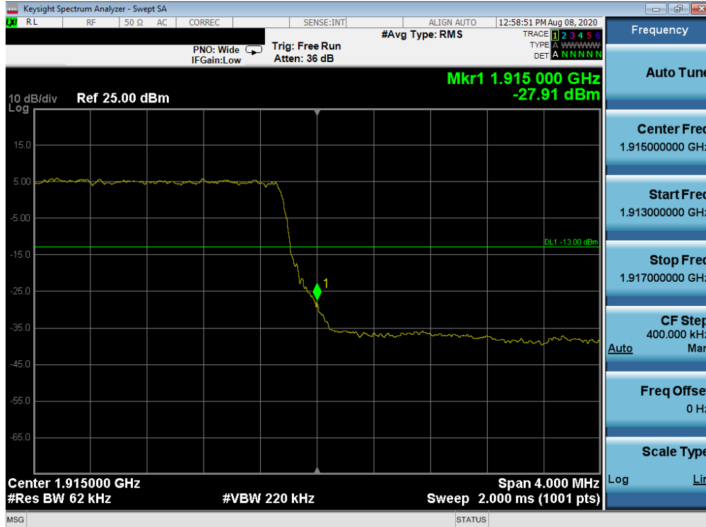
Plot 7-78. Upper Band Edge Plot (LTE Band 25 - 5MHz QPSK – Full RB Configuration)
