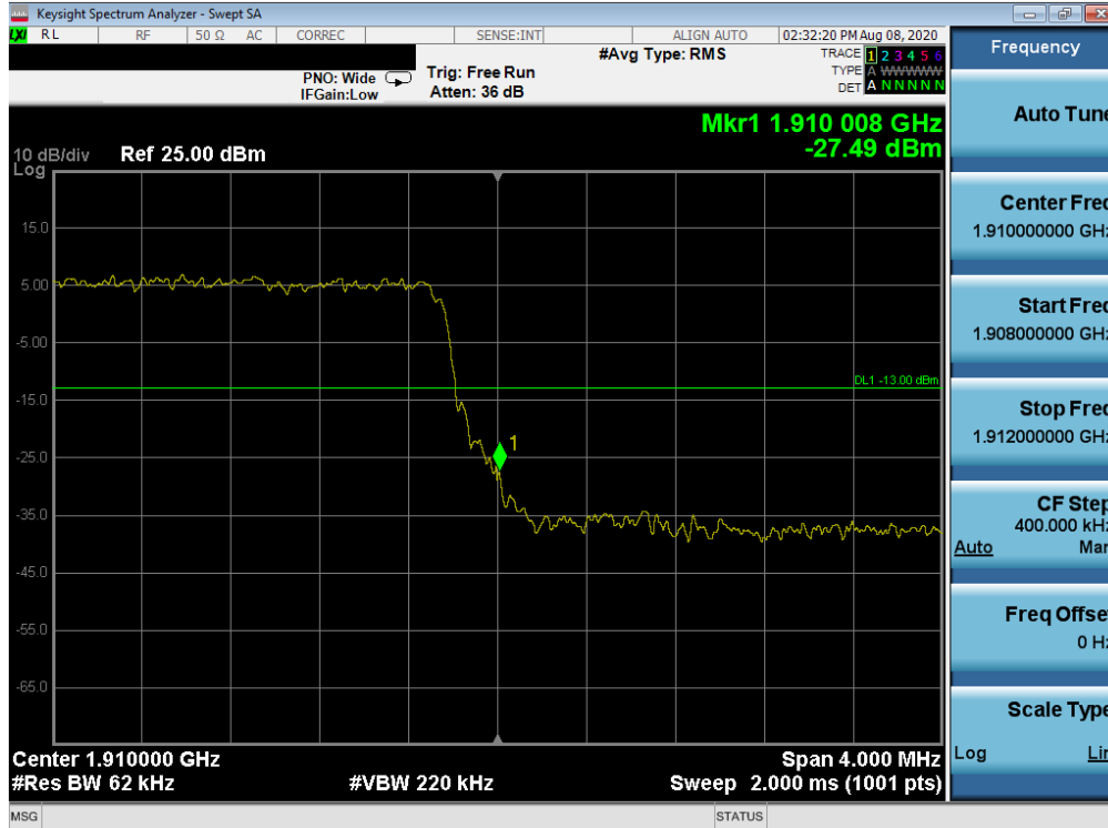
Plot 7-76. Upper Band Edge Plot (LTE Band 2 - 5MHz QPSK – Full RB Configuration)
