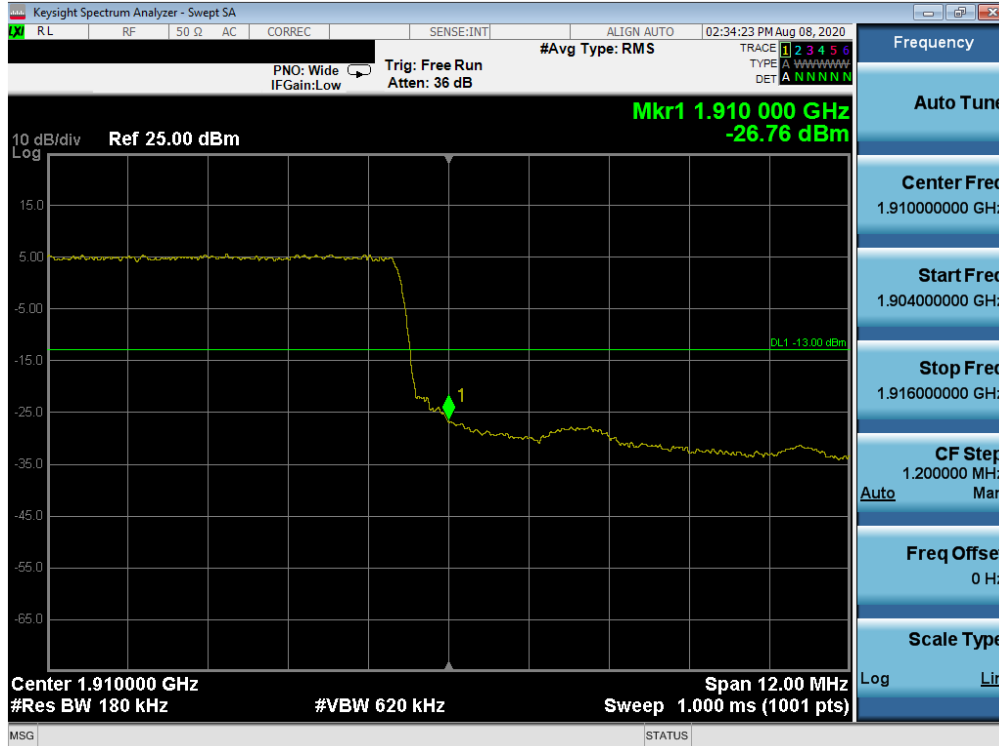
Plot 7-64. Upper Band Edge Plot (LTE Band 2 - 15MHz QPSK – Full RB Configuration)
