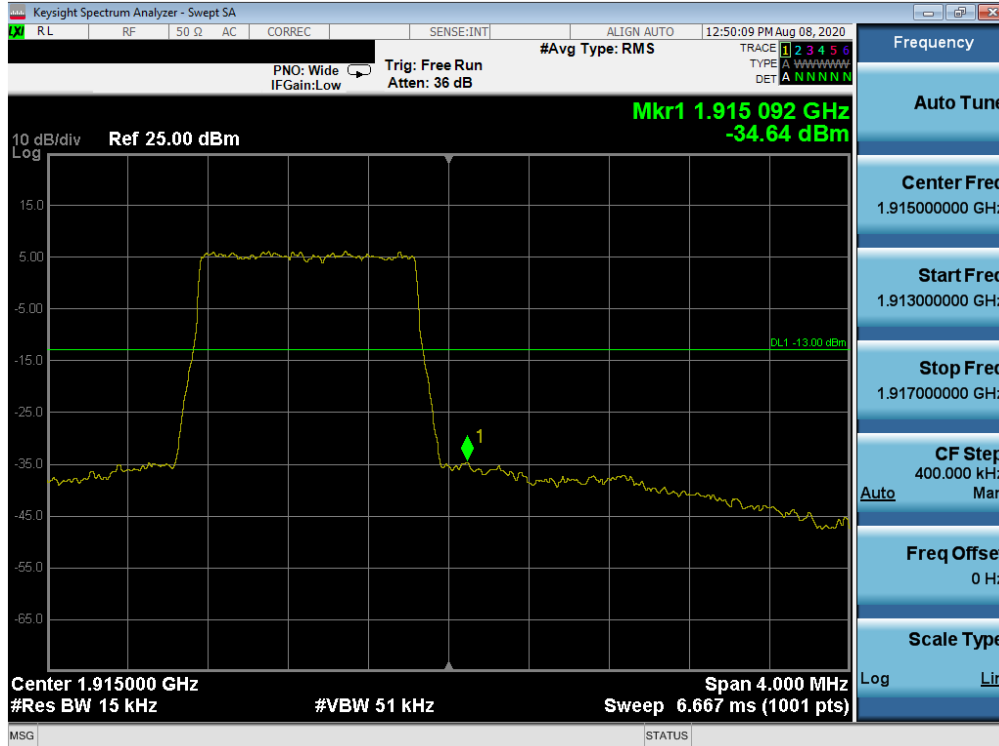
Plot 7-90. Upper Band Edge Plot (LTE Band 25 – 1.4MHz QPSK – Full RB Configuration)
