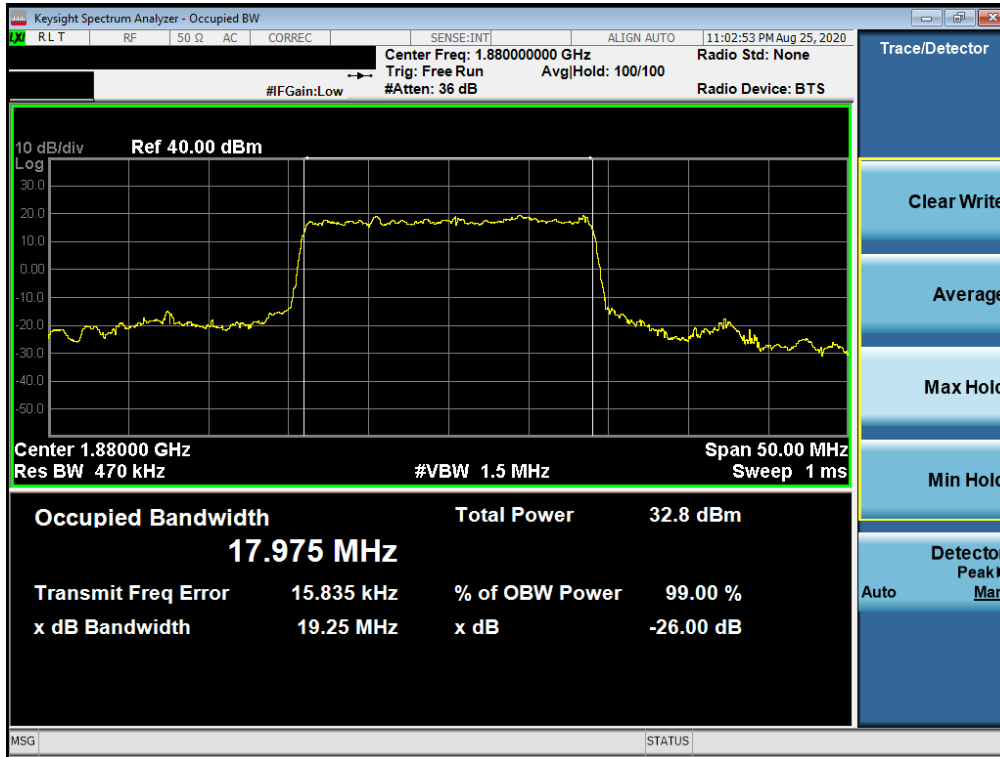
Plot 7-19. Occupied Bandwidth Plot (NR Band n2 - 20.0MHz DFT-s-OFDM BPSK - Full RB)
