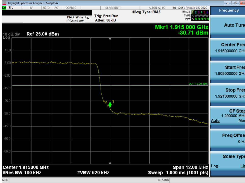
Plot 7-66. Upper Band Edge Plot (LTE Band 25 - 15MHz QPSK – Full RB Configuration)
