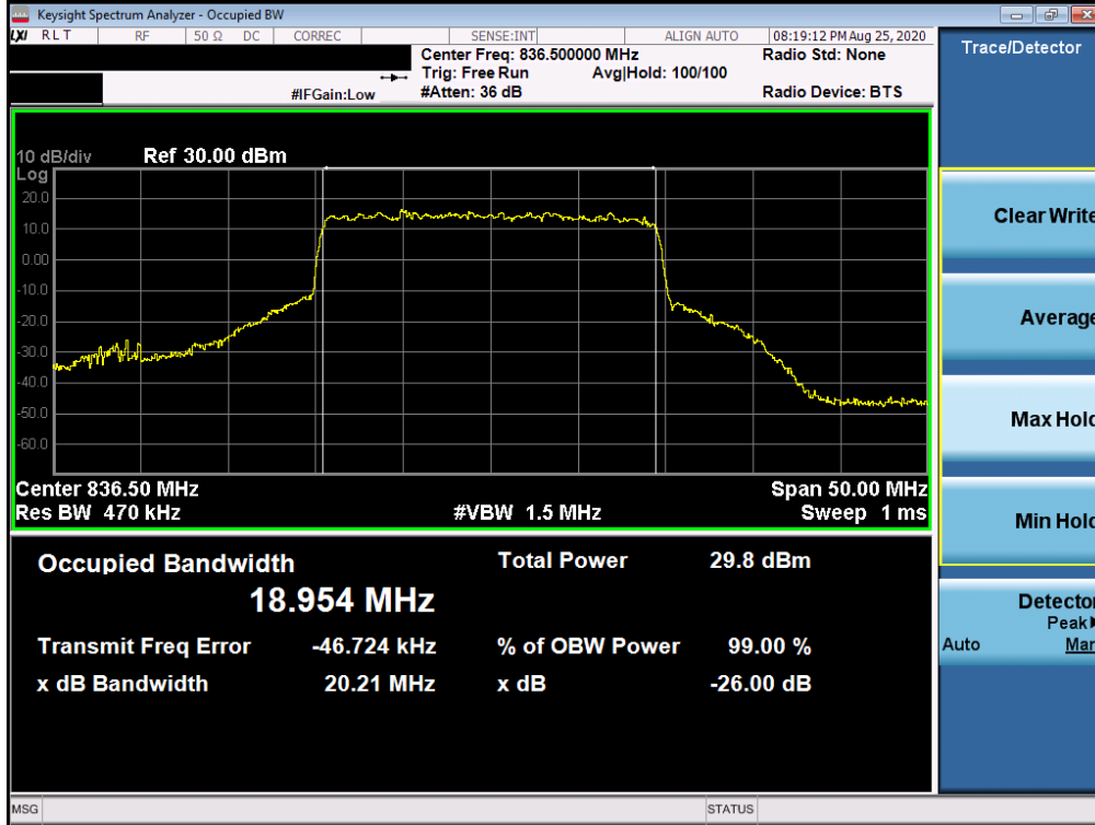
Plot 7-21. Occupied Bandwidth Plot (NR Band n5 - 20MHz 16-QAM - Full RB Configuration)
