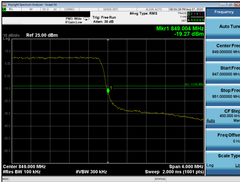
Plot 7-60. Upper Band Edge Plot (LTE Band 26/5 - 3MHz QPSK – Full RB Configuration)
