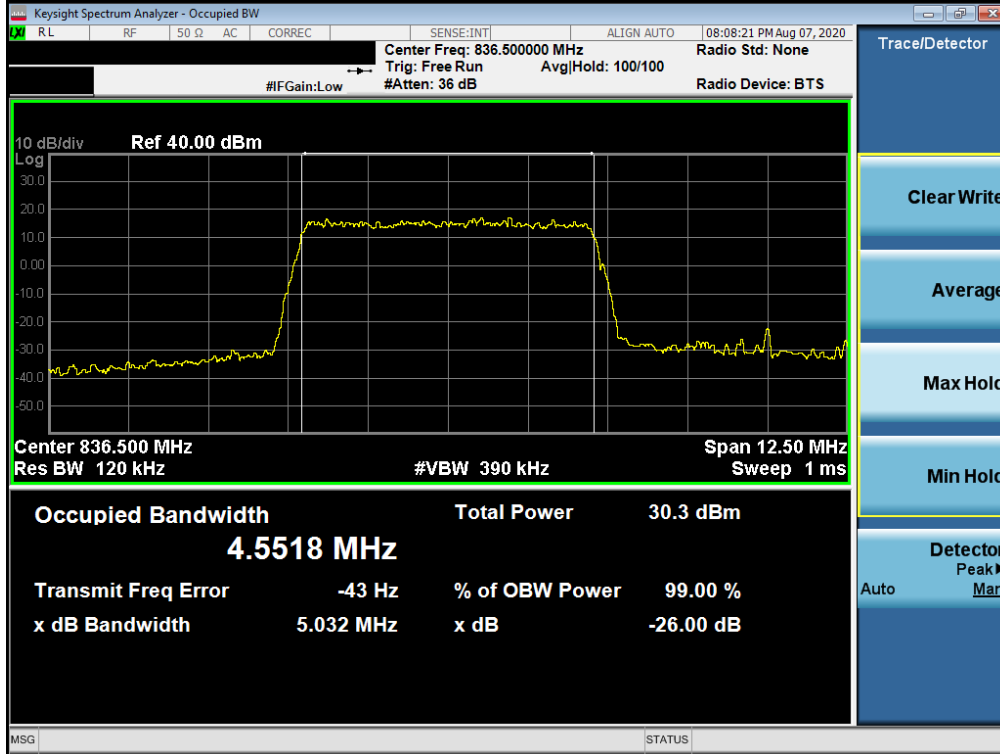
Plot 7-12. Occupied Bandwidth Plot (LTE Band 26/5 - 5MHz 64-QAM - Full RB Configuration)
