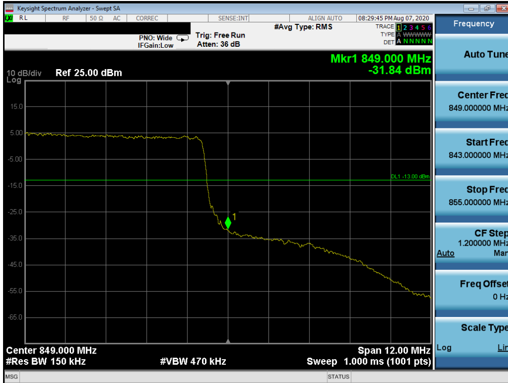
Plot 7-54. Upper Band Edge Plot (LTE Band 26 - 15MHz QPSK – Full RB Configuration)
