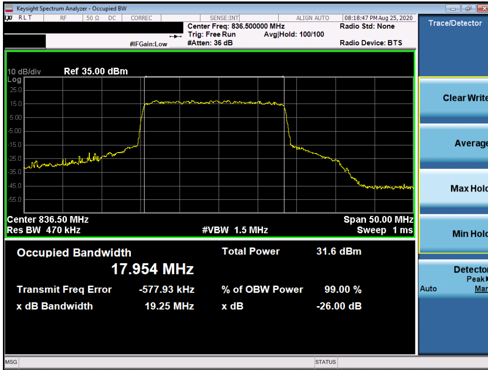
Plot 7-19. Occupied Bandwidth Plot (NR Band n5 - 20MHz \pi/2 BPSK - Full RB Configuration)
