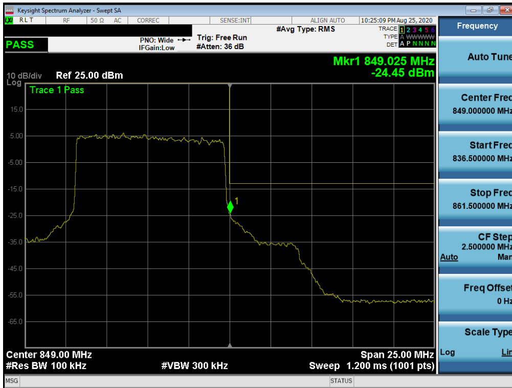
Plot 7-68. Upper Band Edge Plot (NR Band n5 – 10.0MHz - Full RB)
