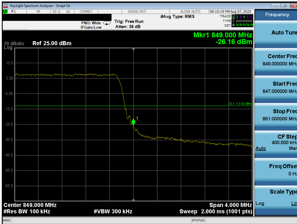
Plot 7-58. Upper Band Edge Plot (LTE Band 26/5 - 5MHz QPSK – Full RB Configuration)
