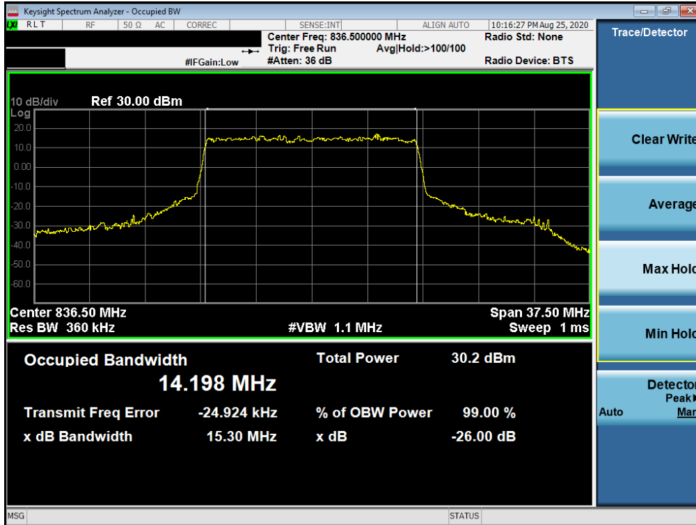
Plot 7-25. Occupied Bandwidth Plot (NR Band n5 - 15MHz 16-QAM - Full RB Configuration)
