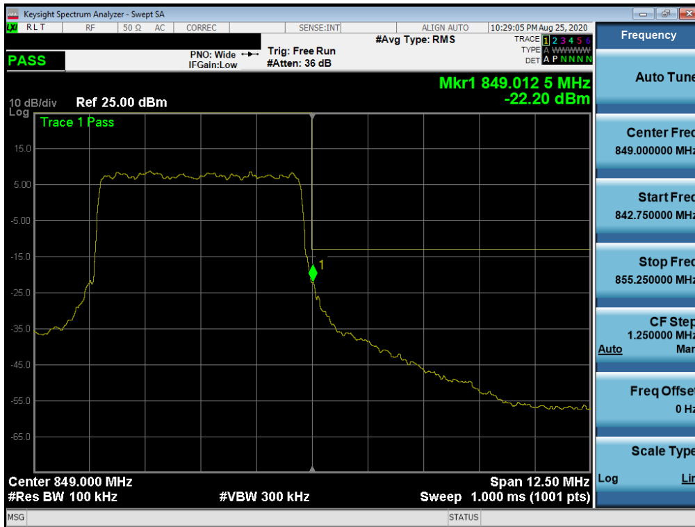
Plot 7-70. Upper Band Edge Plot (NR Band n5 – 5.0MHz - Full RB)
