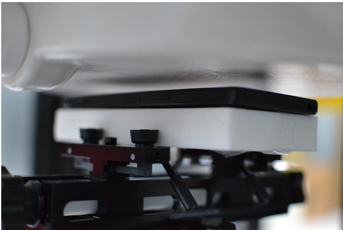
SAR Test Setup Photo 6 – Body-worn/Hotspot, Front Side at 10mm
