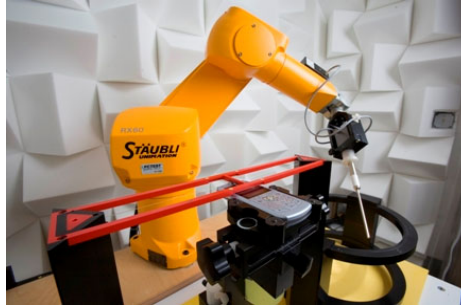
Figure 4-3 SPEAG Robotic System
