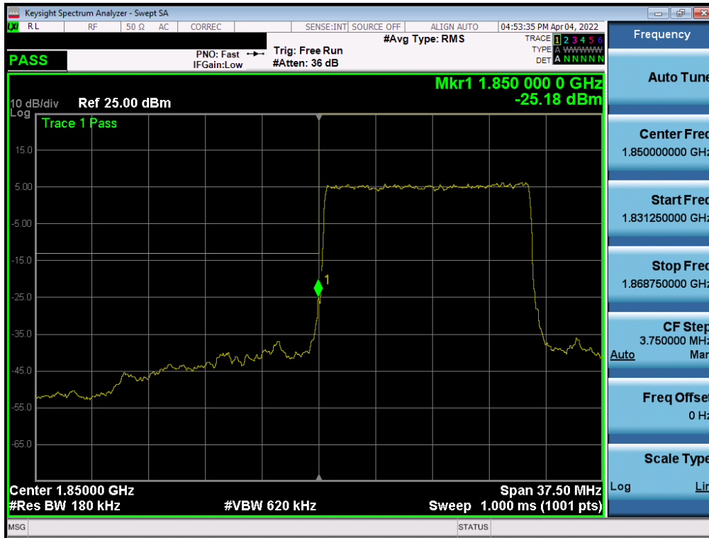
Plot 7-104. Lower Band Edge Plot (NR Band n2 – 15.0MHz - Full RB)
