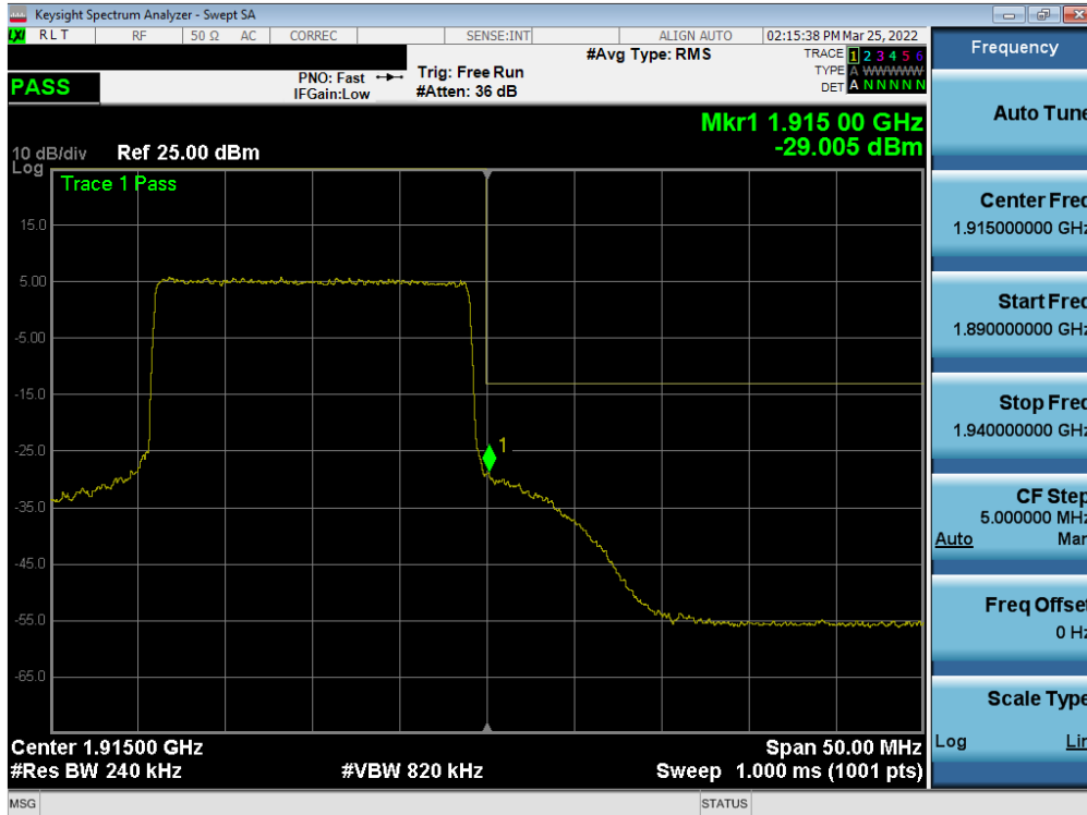
Plot 7-68. Upper Band Edge Plot (LTE Band 25 - 20MHz QPSK – Full RB)
