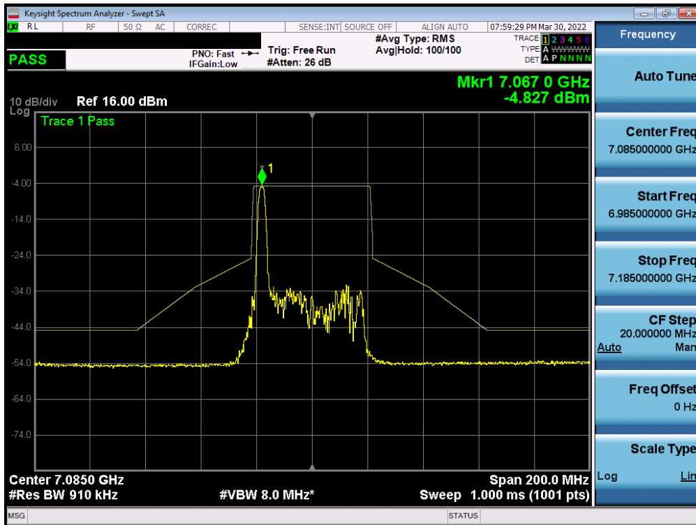
Plot 7-437. In-Band Emission Plot MIMO ANT2 (40MHz BW 802.11ax (26 Tones) (UNII Band 8) – Ch. 227)
