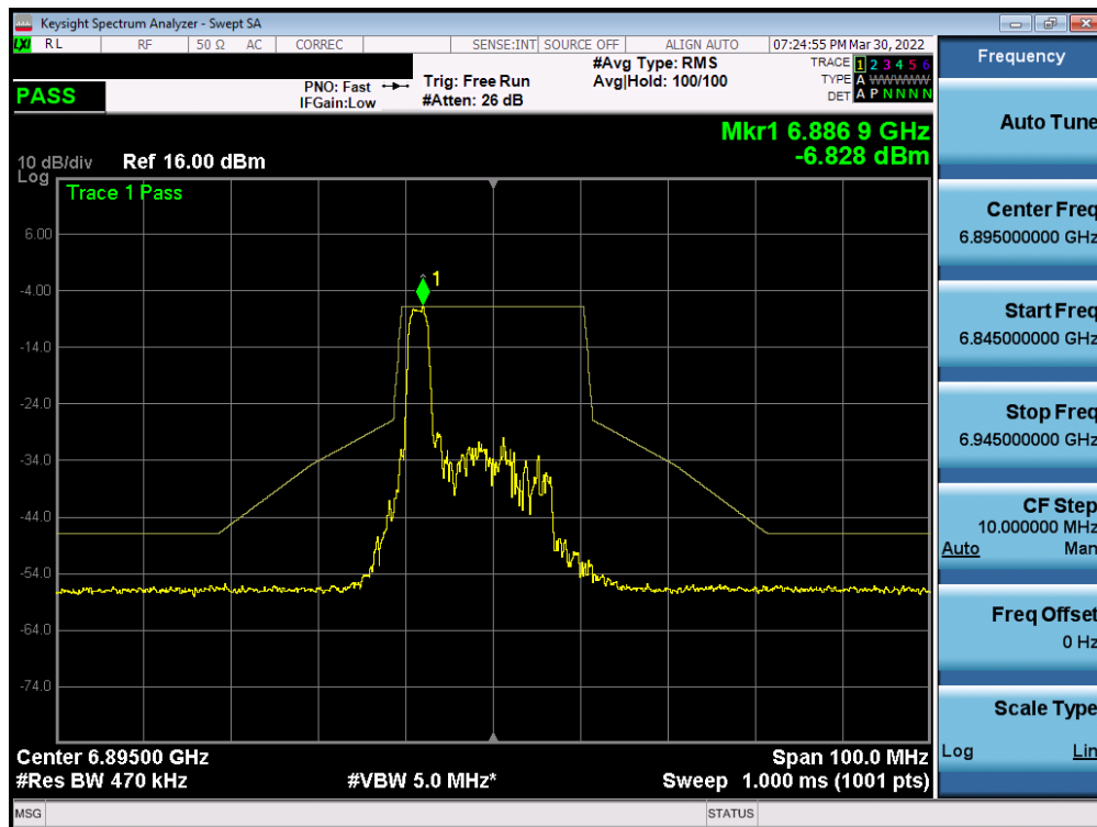
Plot 7-432. In-Band Emission Plot MIMO ANT2 (20MHz BW 802.11ax (26 Tones) (UNII Band 8) – Ch. 189)
