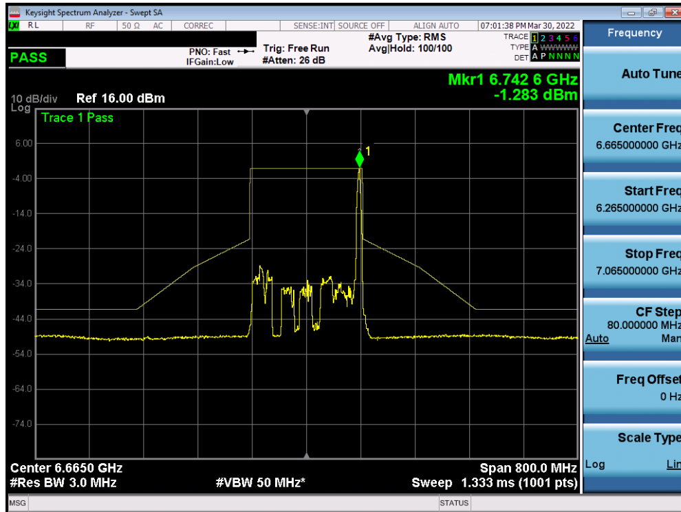
Plot 7-430. In-Band Emission Plot MIMO ANT2 (160MHz BW 802.11ax (26 Tones) (UNII Band 7) – Ch. 143)
