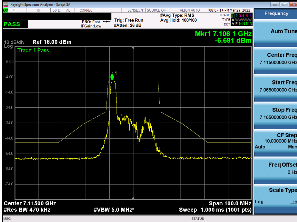
Plot 7-354. In-Band Emission Plot MIMO ANT1 (20MHz BW 802.11ax (26 Tones) (UNII Band 8) – Ch. 233)
