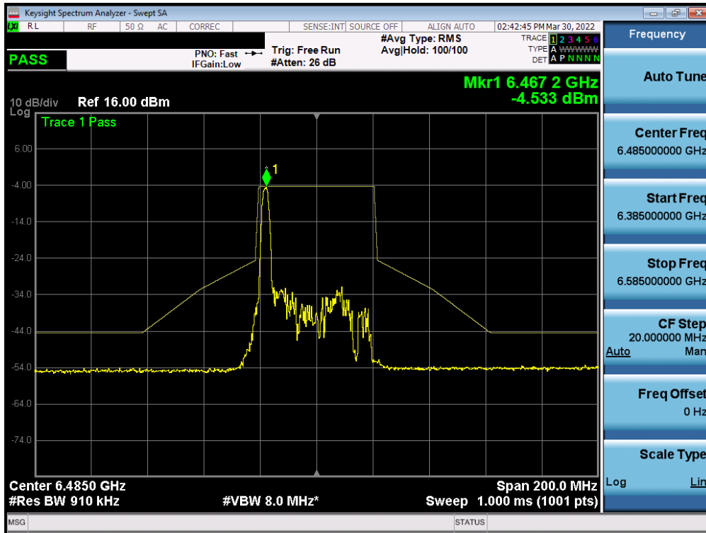
Plot 7-337. In-Band Emission Plot MIMO ANT1 (40MHz BW 802.11ax (26 Tones) (UNII Band 6) – Ch. 107)
