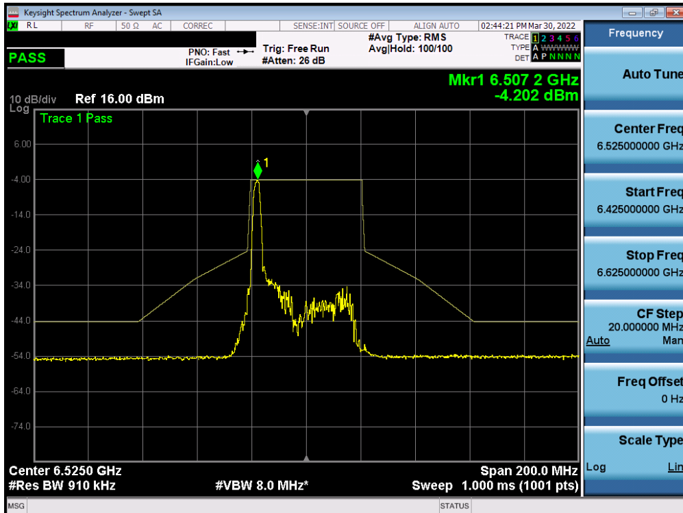
Plot 7-338. In-Band Emission Plot MIMO ANT1 (40MHz BW 802.11ax (26 Tones) (UNII Band 6) – Ch. 115)
