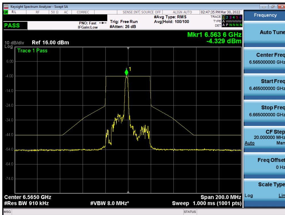
Plot 7-344. In-Band Emission Plot MIMO ANT1 (40MHz BW 802.11ax (26 Tones) (UNII Band 7) – Ch. 123)
