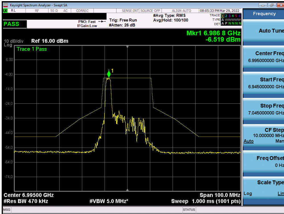
Plot 7-353. In-Band Emission Plot MIMO ANT1 (20MHz BW 802.11ax (26 Tones) (UNII Band 8) – Ch. 209)
