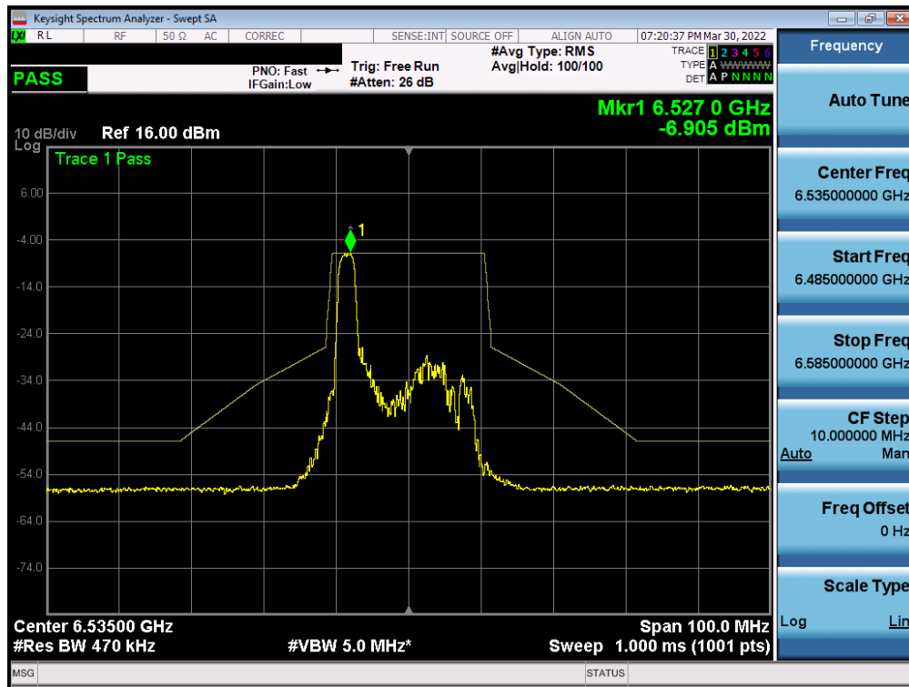
Plot 7-421. In-Band Emission Plot MIMO ANT2 (20MHz BW 802.11ax (26 Tones) (UNII Band 7) – Ch. 117)
