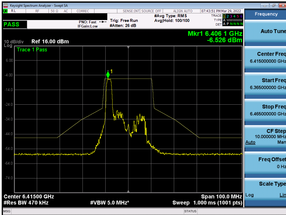
Plot 7-323. In-Band Emission Plot MIMO ANT1 (20MHz BW 802.11ax (26 Tones) UNII Band 5) – Ch. 93)
