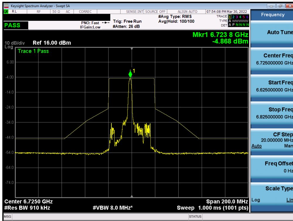
Plot 7-425. In-Band Emission Plot MIMO ANT2 (40MHz BW 802.11ax (26 Tones) (UNII Band 7) – Ch. 155)
