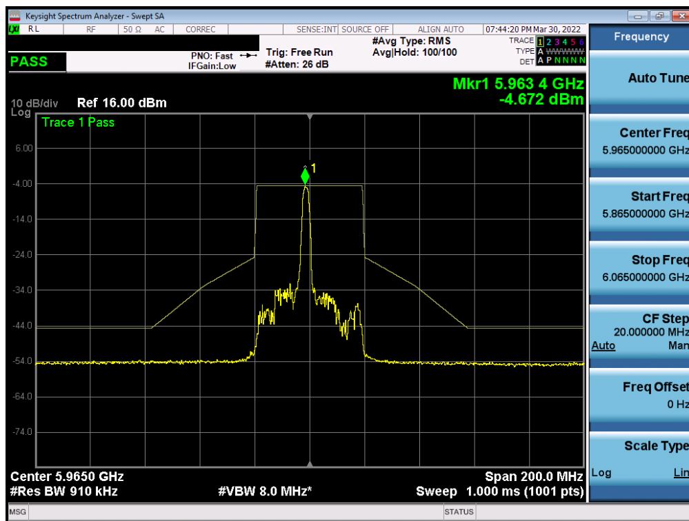
Plot 7-404. In-Band Emission Plot MIMO ANT2 (40MHz BW 802.11ax (26 Tones) (UNII Band 5) – Ch. 3)
