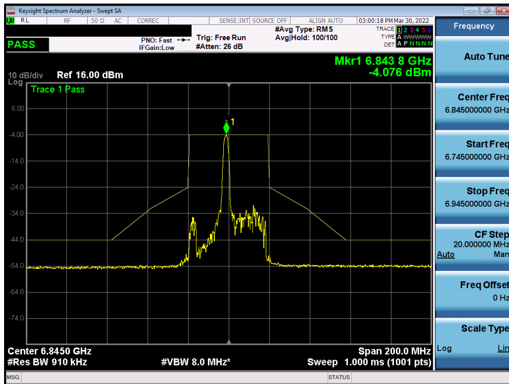
Plot 7-346. In-Band Emission Plot MIMO ANT1 (40MHz BW 802.11ax (26 Tones) (UNII Band 7) – Ch. 179)
