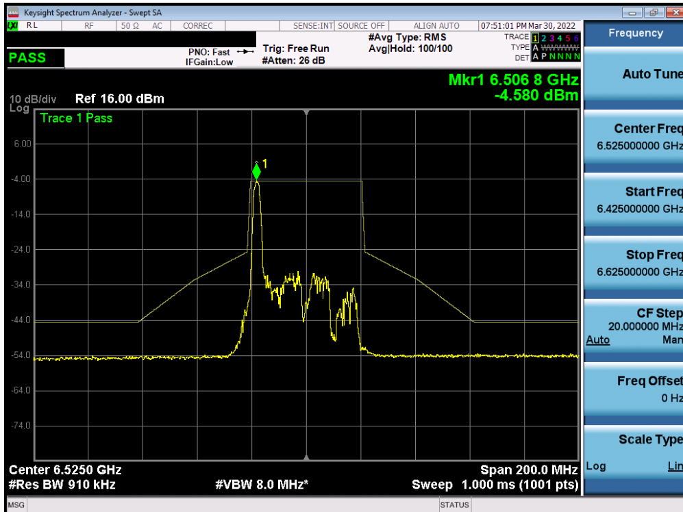
Plot 7-418. In-Band Emission Plot MIMO ANT2 (40MHz BW 802.11ax (26 Tones) (UNII Band 6) – Ch. 115)
