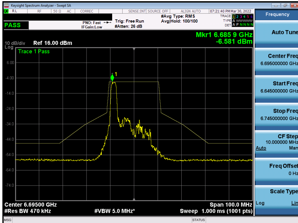
Plot 7-422. In-Band Emission Plot MIMO ANT2 (20MHz BW 802.11ax (26 Tones) (UNII Band 7) – Ch. 149)
