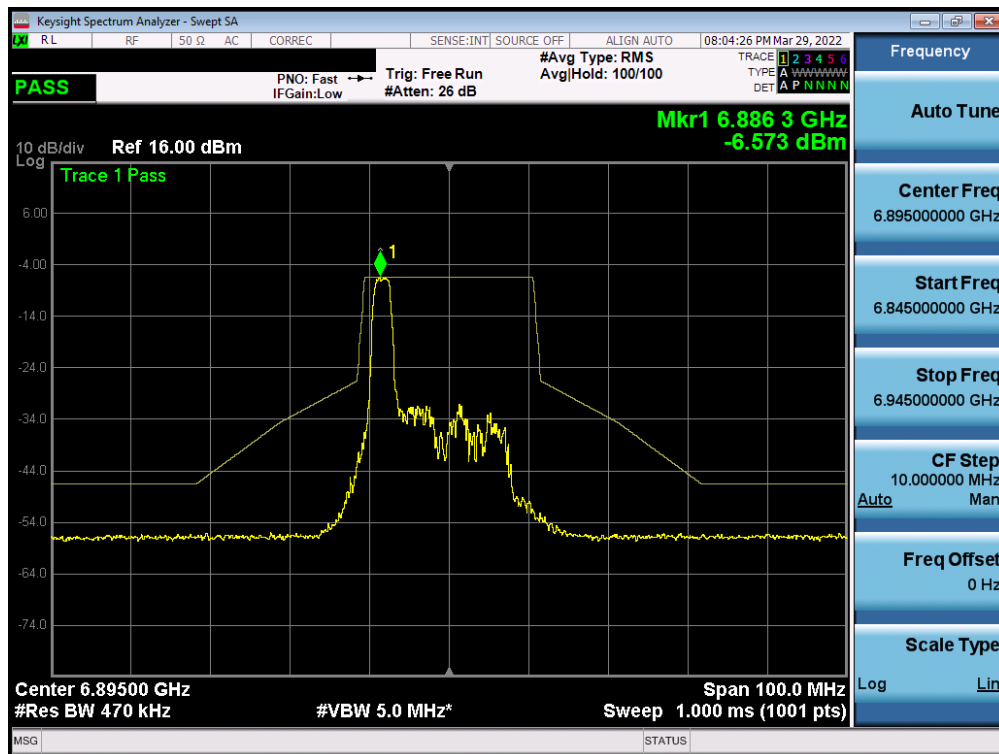
Plot 7-352. In-Band Emission Plot MIMO ANT1 (20MHz BW 802.11ax (26 Tones) (UNII Band 8) – Ch. 189)
