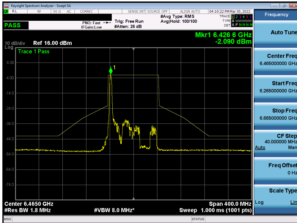
Plot 7-339. In-Band Emission Plot MIMO ANT1 (80MHz BW 802.11ax (26 Tones) (UNII Band 6) – Ch. 103)
