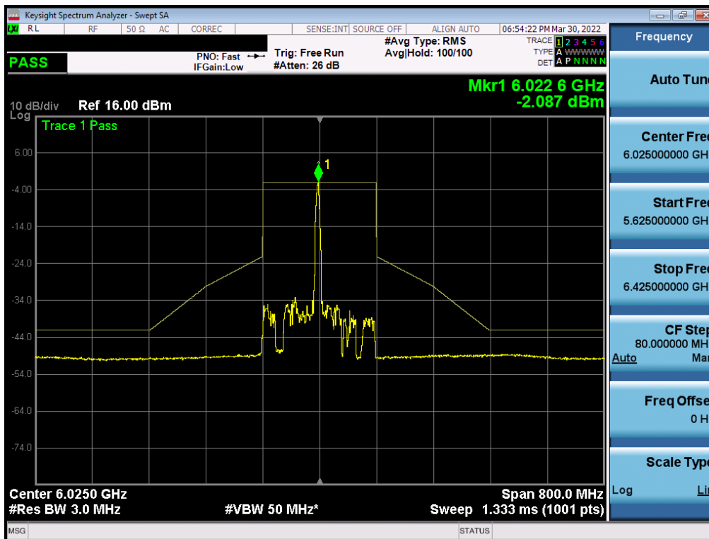
Plot 7-410. In-Band Emission Plot MIMO ANT2 (160MHz BW 802.11ax (26 Tones) (UNII Band 5) – Ch. 15)
