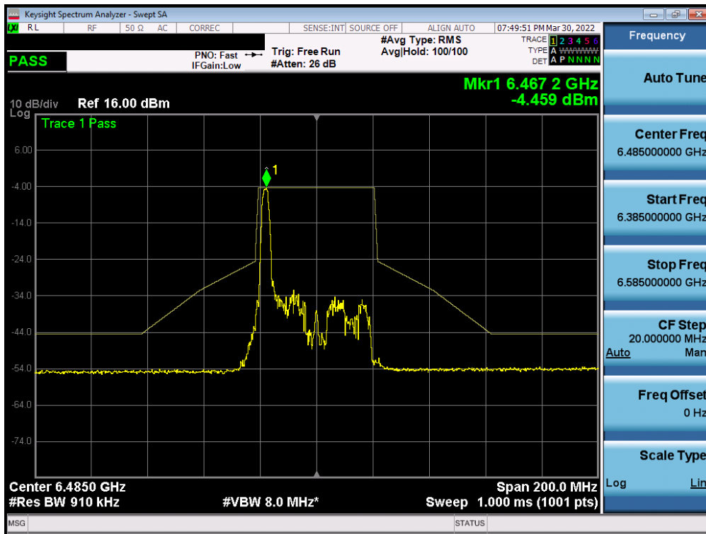
Plot 7-417. In-Band Emission Plot MIMO ANT2 (40MHz BW 802.11ax (26 Tones) (UNII Band 6) – Ch. 107)
