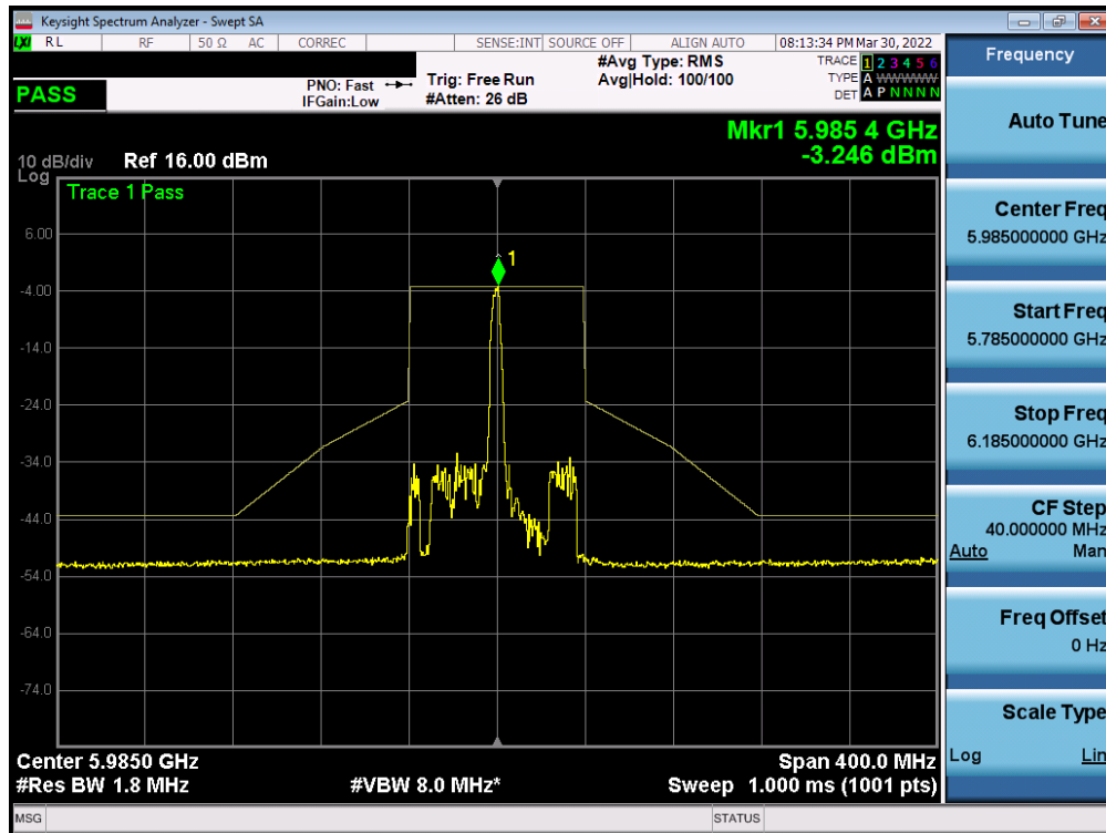
Plot 7-407. In-Band Emission Plot MIMO ANT2 (80MHz BW 802.11ax (26 Tones) (UNII Band 5) – Ch. 7)
