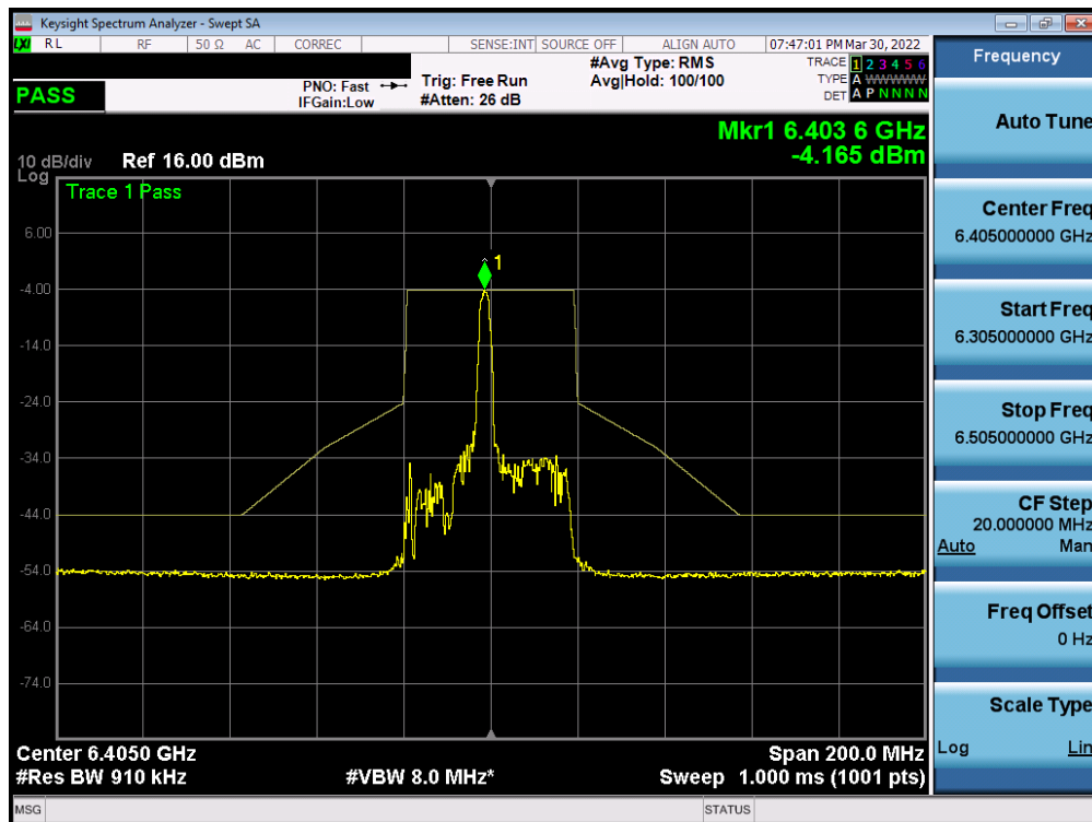
Plot 7-406. In-Band Emission Plot MIMO ANT2 (40MHz BW 802.11ax (26 Tones) (UNII Band 5) – Ch. 91)
