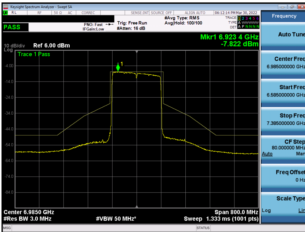
Plot 7-400. In-Band Emission Plot MIMO ANT1 (160MHz BW 802.11ax (Full Tones) (UNII Band 8) – Ch. 207)
