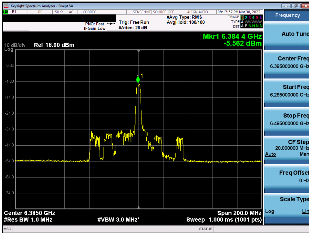
Plot 7-249. Power Spectral Density Plot MIMO ANT2 (80MHz BW 802.11ax (26 Tones) (UNII Band 5) – Ch. 87)
