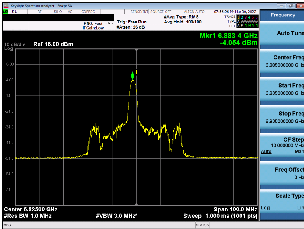
Plot 7-275. Power Spectral Density Plot MIMO ANT2 (40MHz BW 802.11ax (26 Tones) (UNII Band 8) – Ch. 187)
