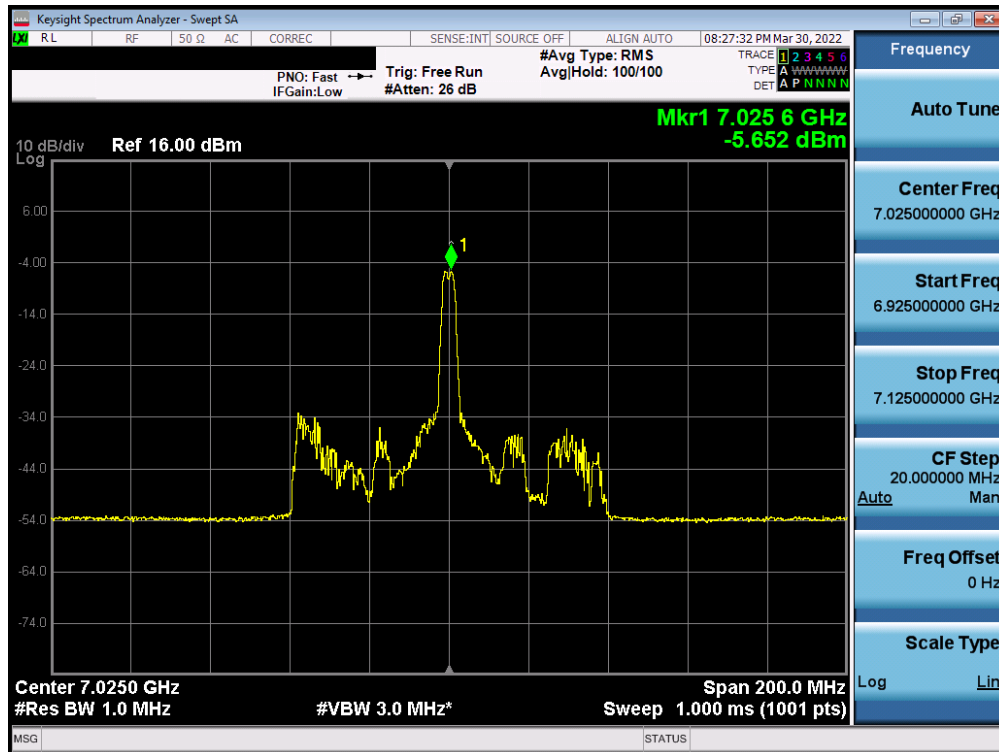
Plot 7-279. Power Spectral Density Plot MIMO ANT2 (80MHz BW 802.11ax (26 Tones) (UNII Band 8) – Ch. 215)
