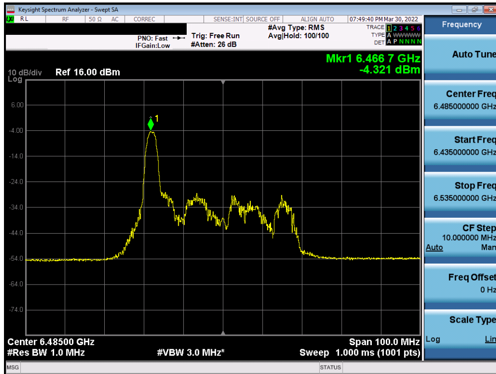
Plot 7-257. Power Spectral Density Plot MIMO ANT2 (40MHz BW 802.11ax (26 Tones) (UNII Band 6) – Ch. 107)
