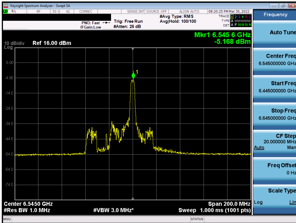
Plot 7-267. Power Spectral Density Plot MIMO ANT2 (80MHz BW 802.11ax (26 Tones) (UNII Band 7) – Ch. 119)
