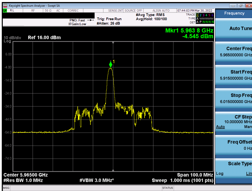
Plot 7-244. Power Spectral Density Plot MIMO ANT2 (40MHz BW 802.11ax (26 Tones) (UNII Band 5) – Ch. 3)
