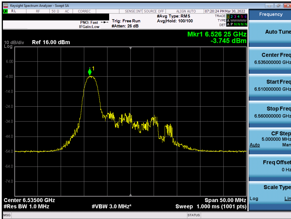
Plot 7-261. Power Spectral Density Plot MIMO ANT2 (20MHz BW 802.11ax (26 Tones) (UNII Band 7) – Ch. 117)
