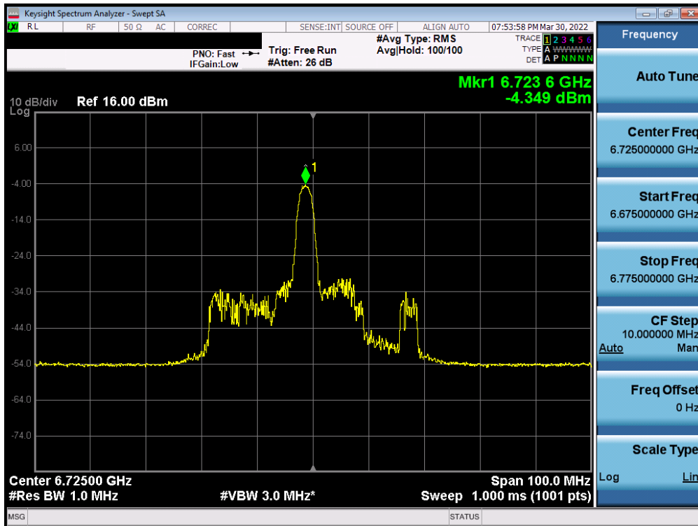
Plot 7-265. Power Spectral Density Plot MIMO ANT2 (40MHz BW 802.11ax (26 Tones) (UNII Band 7) – Ch. 155)
