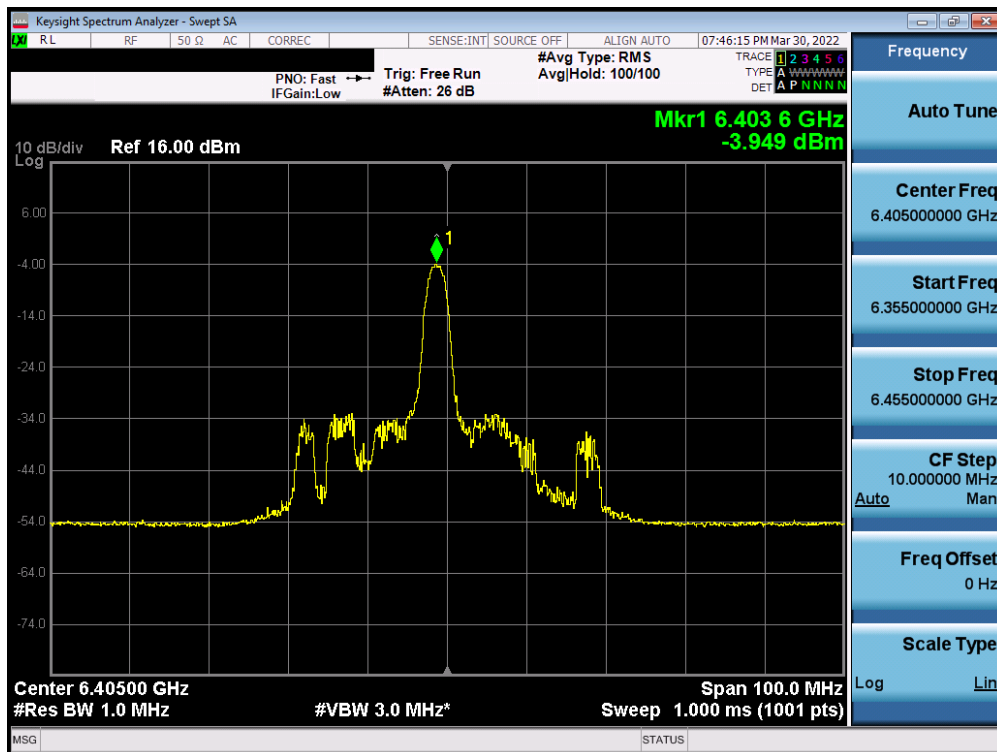
Plot 7-246. Power Spectral Density Plot MIMO ANT2 (40MHz BW 802.11ax (26 Tones) (UNII Band 5) – Ch. 91)
