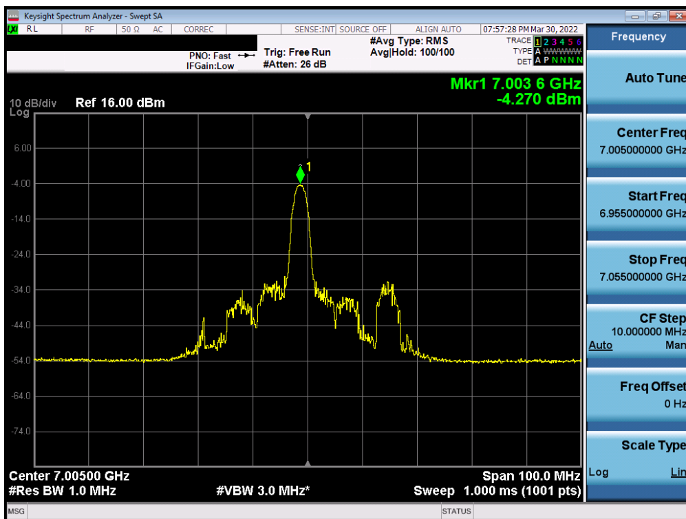
Plot 7-276. Power Spectral Density Plot MIMO ANT2 (40MHz BW 802.11ax (26 Tones) (UNII Band 8) – Ch. 211)
