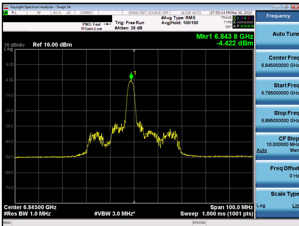
Plot 7-266. Power Spectral Density Plot MIMO ANT2 (40MHz BW 802.11ax (26 Tones) (UNII Band 7) – Ch. 179)
