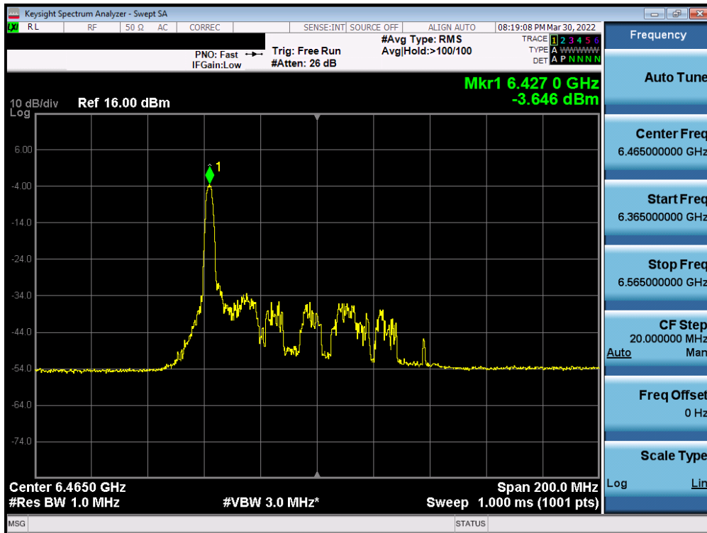
Plot 7-259. Power Spectral Density Plot MIMO ANT2 (80MHz BW 802.11ax (26 Tones) (UNII Band 6) – Ch. 103)
