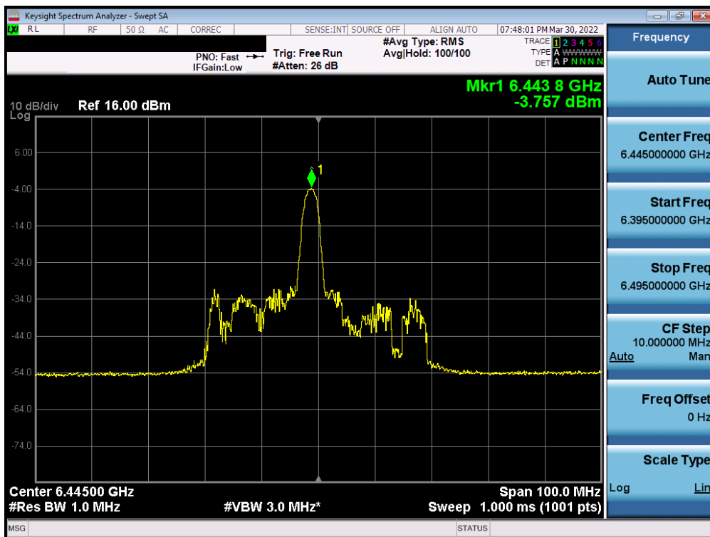
Plot 7-256. Power Spectral Density Plot MIMO ANT2 (40MHz BW 802.11ax (26 Tones) (UNII Band 6) – Ch. 99)
