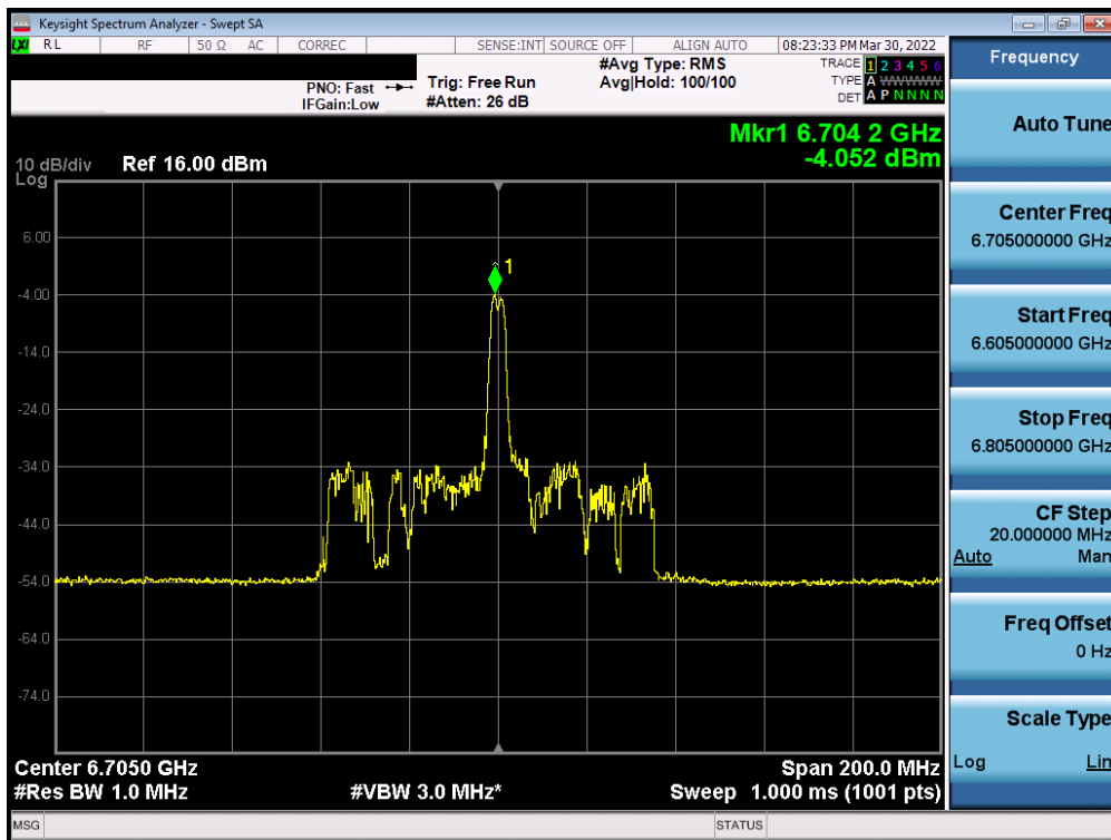
Plot 7-268. Power Spectral Density Plot MIMO ANT2 (80MHz BW 802.11ax (26 Tones) (UNII Band 7) – Ch. 151)
