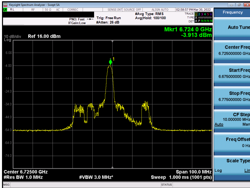
Plot 7-185. Power Spectral Density Plot MIMO ANT1 (40MHz BW 802.11ax (26 Tones) (UNII Band 7) – Ch. 155)
