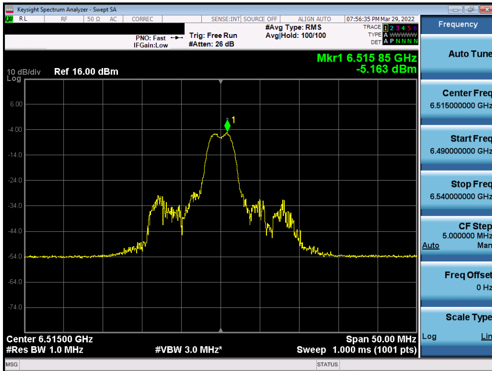
Plot 7-175. Power Spectral Density Plot MIMO ANT1 (20MHz BW 802.11ax (26 Tones) (UNII Band 6) – Ch. 113)
