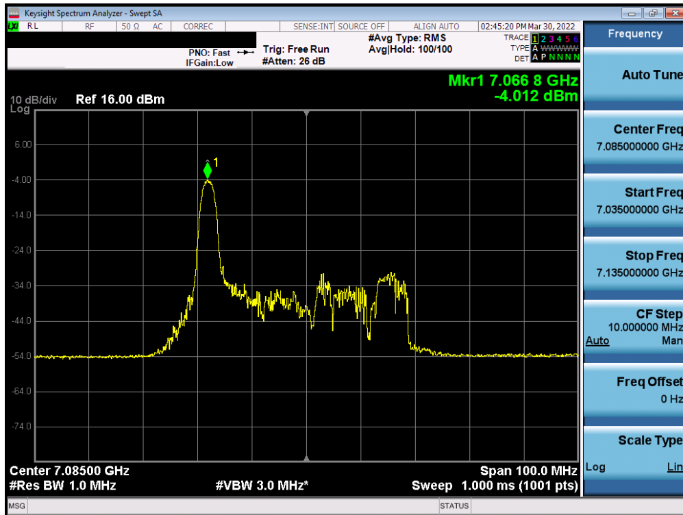
Plot 7-197. Power Spectral Density Plot MIMO ANT1 (40MHz BW 802.11ax (26 Tones) (UNII Band 8) – Ch. 227)
