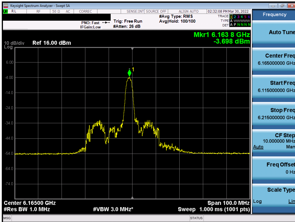
Plot 7-165. Power Spectral Density Plot MIMO ANT1 (40MHz BW 802.11ax (26 Tones) (UNII Band 5) – Ch. 43)
