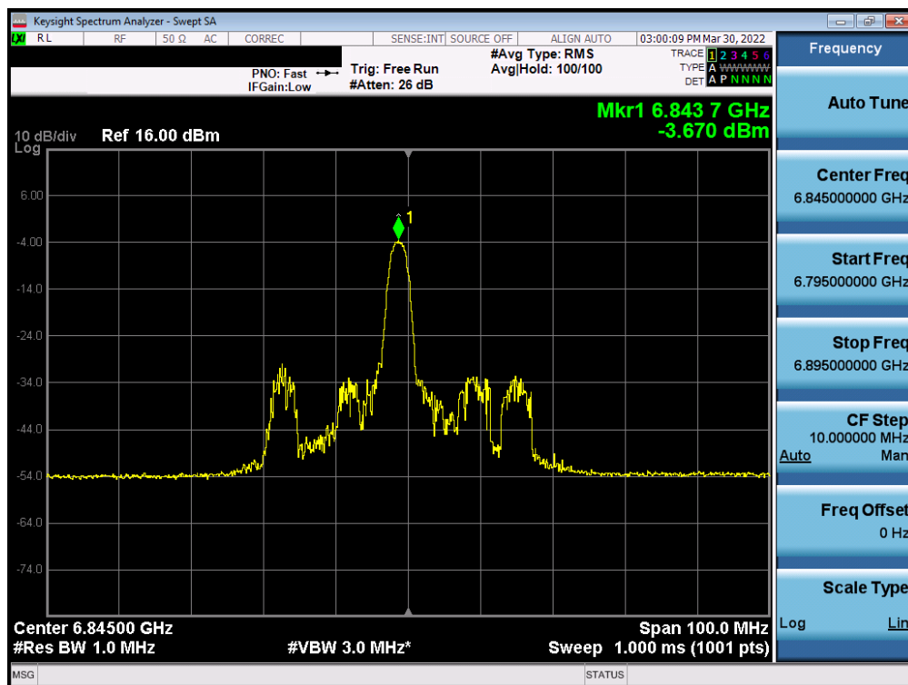
Plot 7-186. Power Spectral Density Plot MIMO ANT1 (40MHz BW 802.11ax (26 Tones) (UNII Band 7) – Ch. 179)
