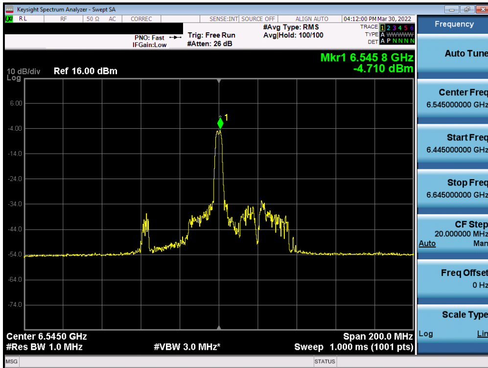
Plot 7-187. Power Spectral Density Plot MIMO ANT1 (80MHz BW 802.11ax (26 Tones) (UNII Band 7) – Ch. 119)
