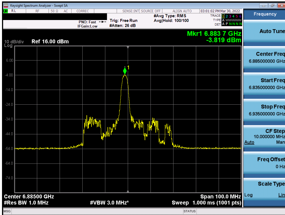
Plot 7-195. Power Spectral Density Plot MIMO ANT1 (40MHz BW 802.11ax (26 Tones) (UNII Band 8) – Ch. 187)
