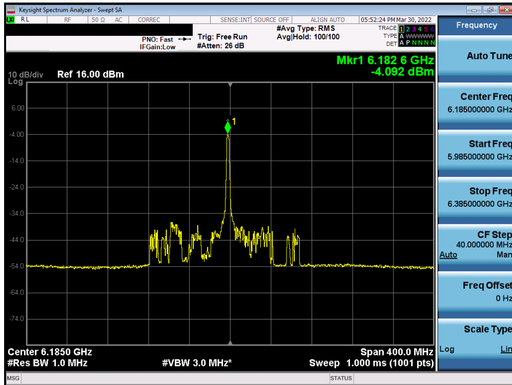
Plot 7-171. Power Spectral Density Plot MIMO ANT1 (160MHz BW 802.11ax (26 Tones) (UNII Band 5) – Ch. 47)
