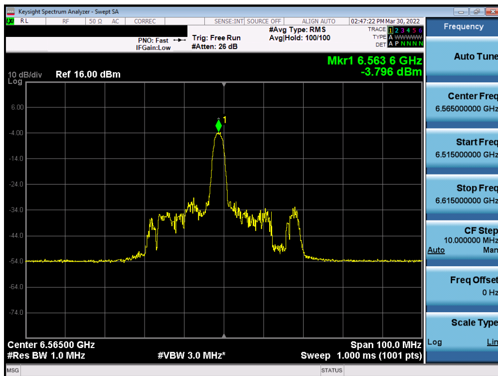
Plot 7-184. Power Spectral Density Plot MIMO ANT1 (40MHz BW 802.11ax (26 Tones) (UNII Band 7) – Ch. 123)
