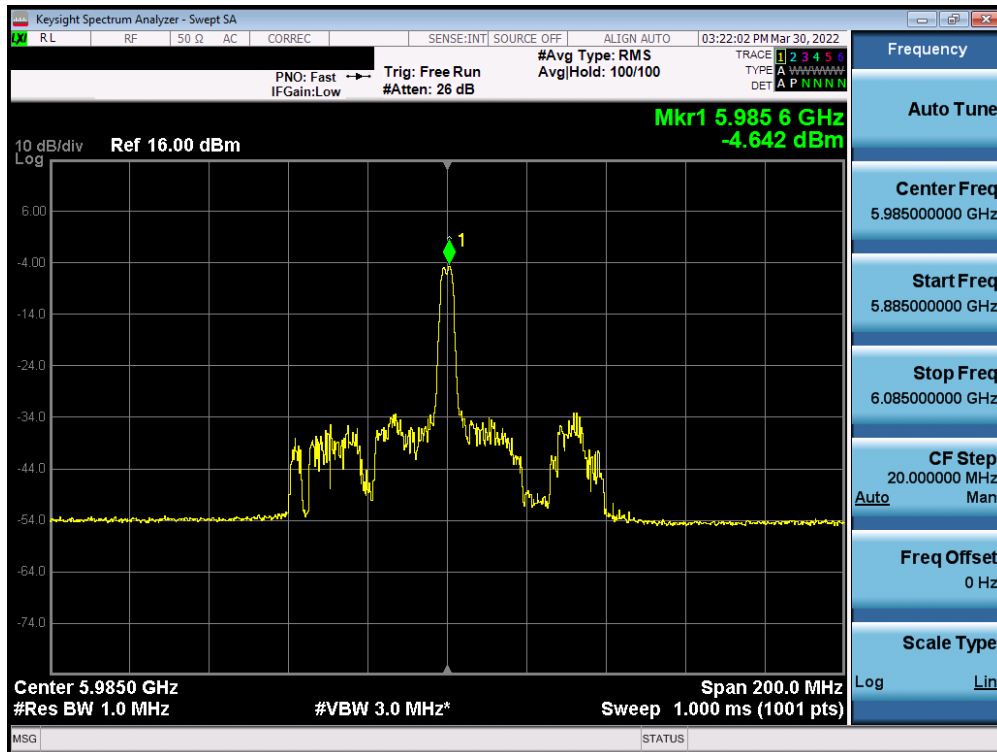
Plot 7-167. Power Spectral Density Plot MIMO ANT1 (80MHz BW 802.11ax (26 Tones) (UNII Band 5) – Ch. 7)
