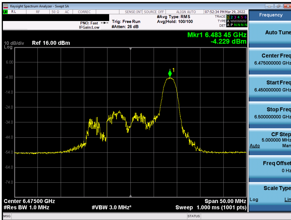
Plot 7-174. Power Spectral Density Plot MIMO ANT1 (20MHz BW 802.11ax (26 Tones) (UNII Band 6) – Ch. 105)
