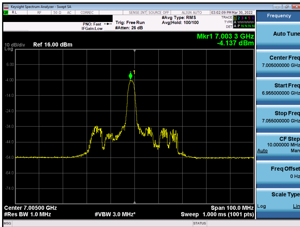
Plot 7-196. Power Spectral Density Plot MIMO ANT1 (40MHz BW 802.11ax (26 Tones) (UNII Band 8) – Ch. 211)
