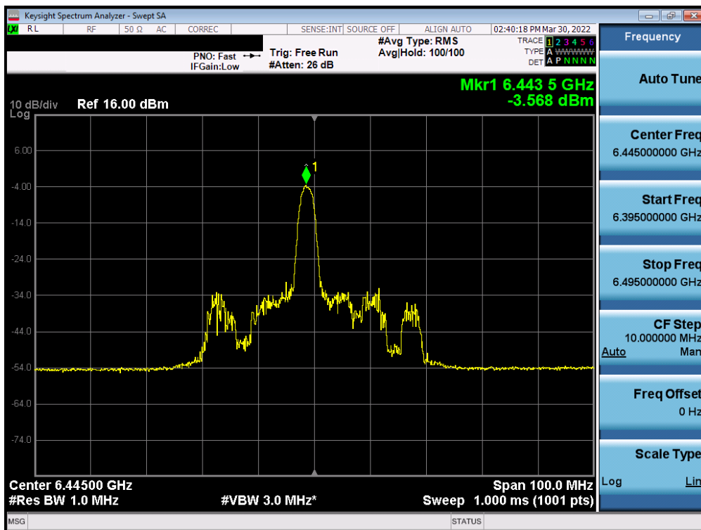
Plot 7-176. Power Spectral Density Plot MIMO ANT1 (40MHz BW 802.11ax (26 Tones) (UNII Band 6) – Ch. 99)
