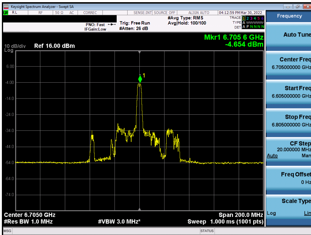
Plot 7-188. Power Spectral Density Plot MIMO ANT1 (80MHz BW 802.11ax (26 Tones) (UNII Band 7) – Ch. 151)
