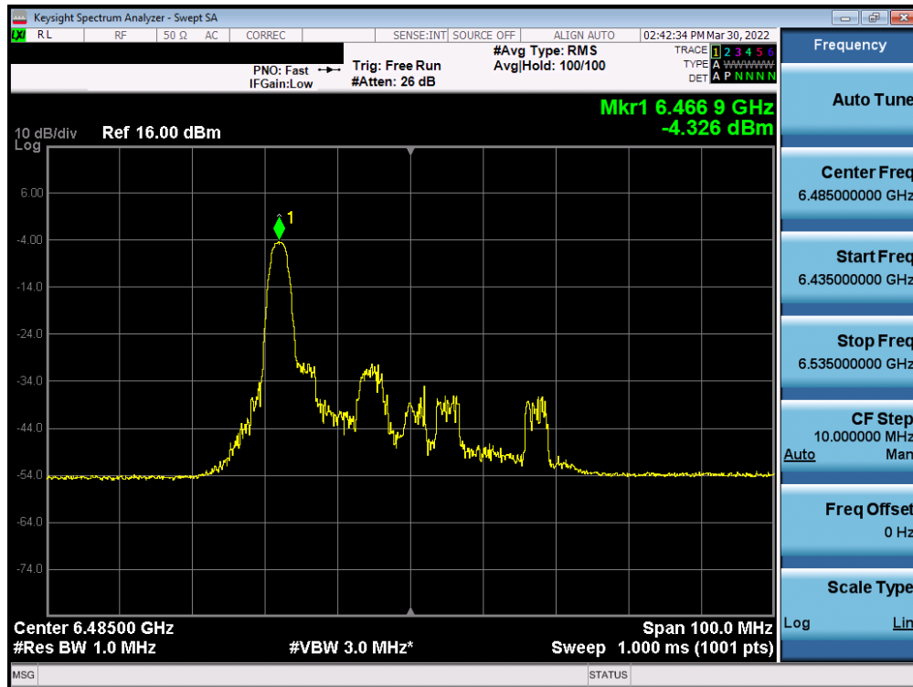
Plot 7-177. Power Spectral Density Plot MIMO ANT1 (40MHz BW 802.11ax (26 Tones) (UNII Band 6) – Ch. 107)
