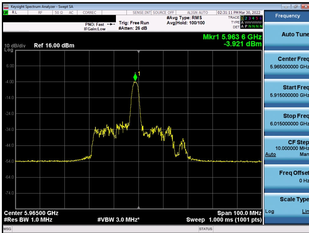
Plot 7-164. Power Spectral Density Plot MIMO ANT1 (40MHz BW 802.11ax (26 Tones) (UNII Band 5) – Ch. 3)
