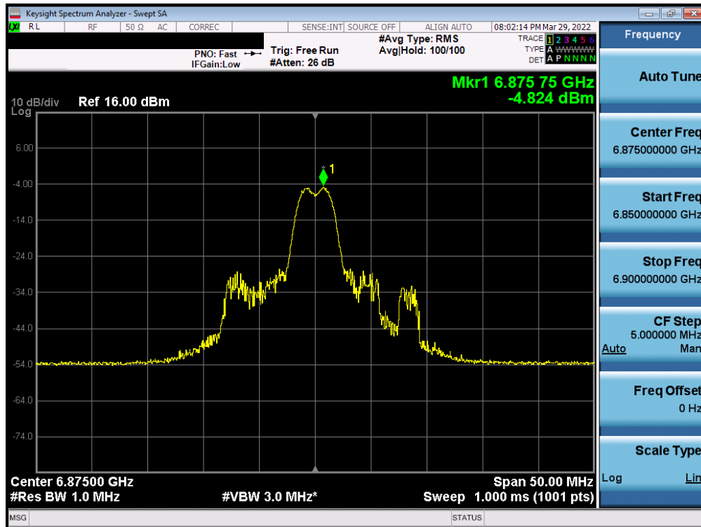
Plot 7-183. Power Spectral Density Plot MIMO ANT1 (20MHz BW 802.11ax (26 Tones) (UNII Band 7) – Ch. 185)
