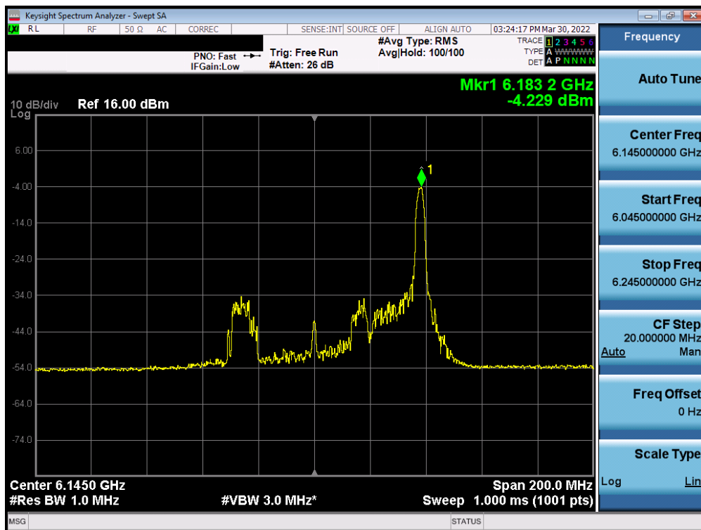
Plot 7-168. Power Spectral Density Plot MIMO ANT1 (80MHz BW 802.11ax (26 Tones) (UNII Band 5) – Ch. 39)
