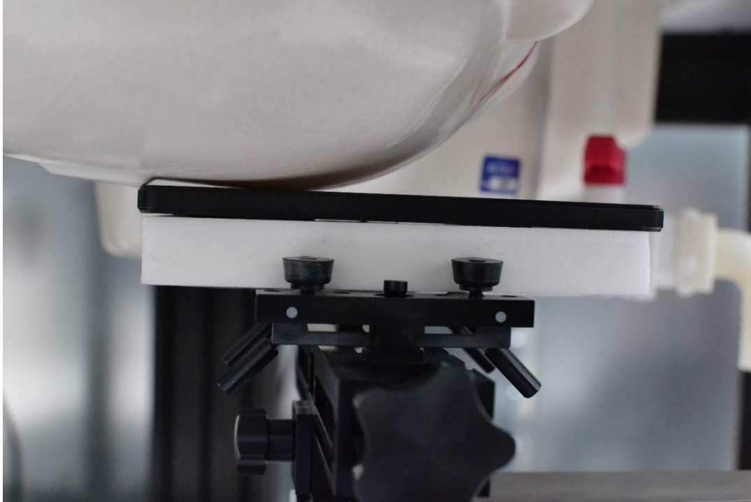
Figure F-3 SAR Test Setup Photo – Head Right, Cheek at 0 mm
