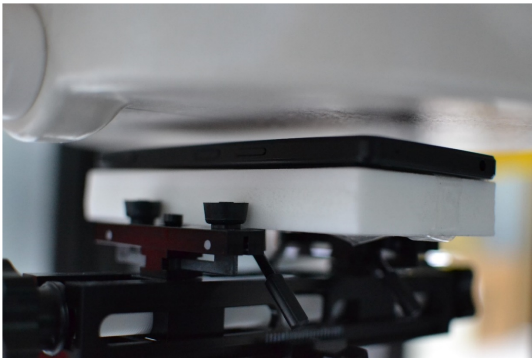
Figure F-9 SAR Test Setup Photo – Bodyworn, Front Side at 10 mm
