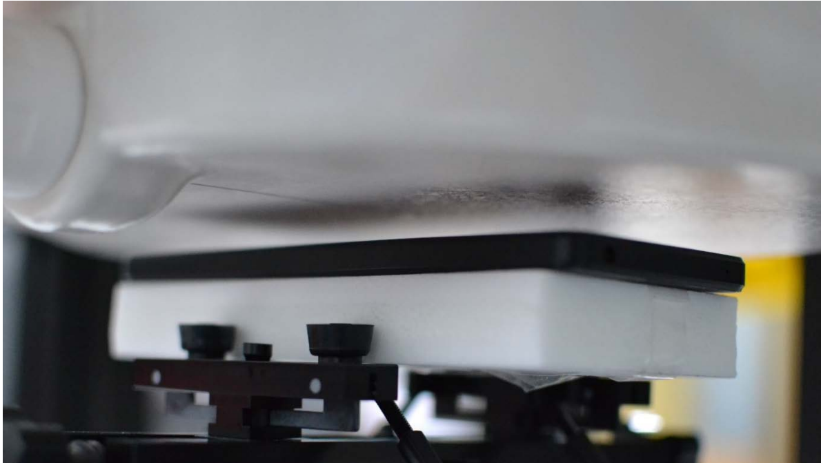
Figure F-7 SAR Test Setup Photo – Bodyworn, Back Side at 10 mm
