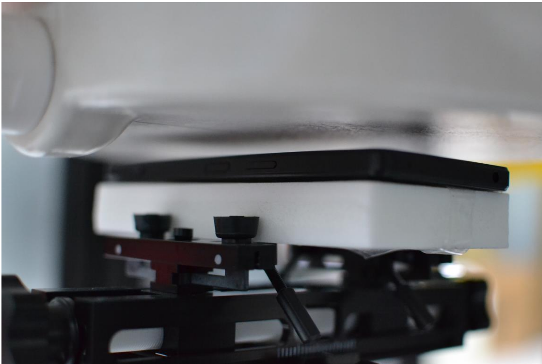
Test Setup Photo 7 – Body, Front Side, 10 mm
