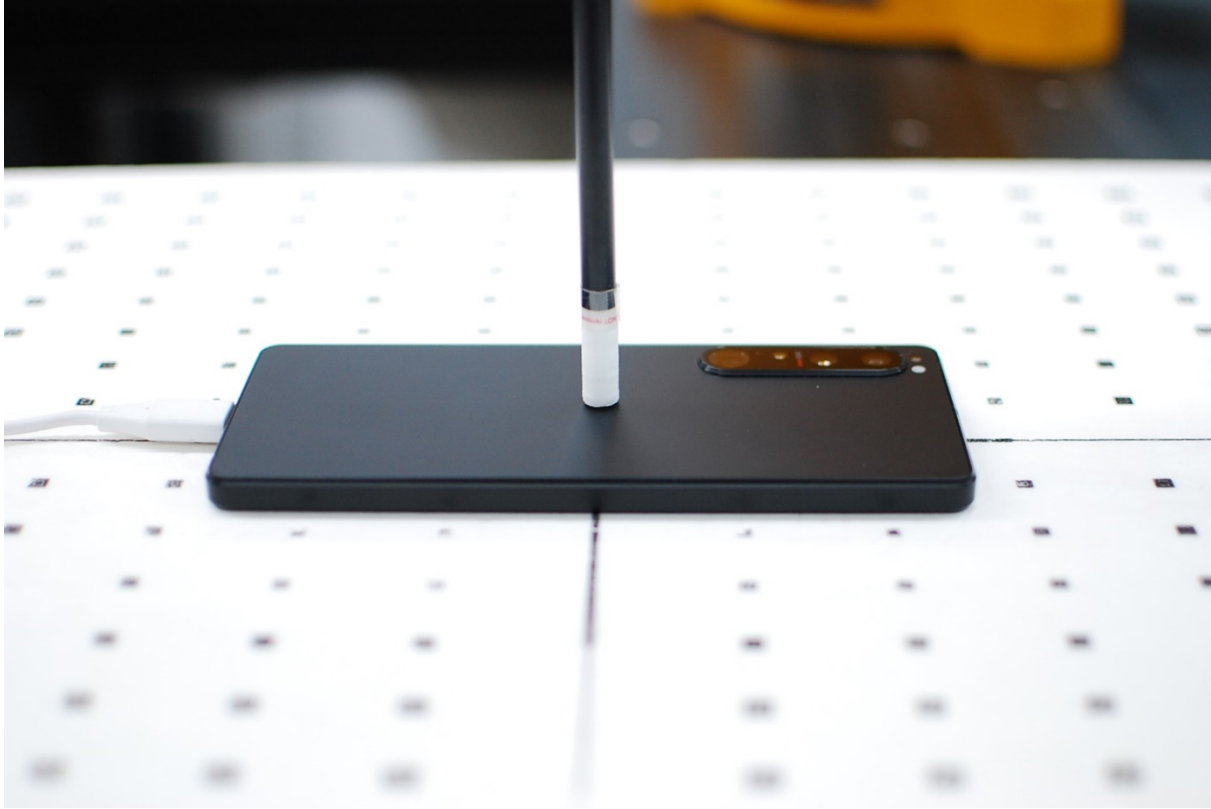
Figure E-3 Near Field Power Density Test Setup Photo – Back Side at 2 mm
