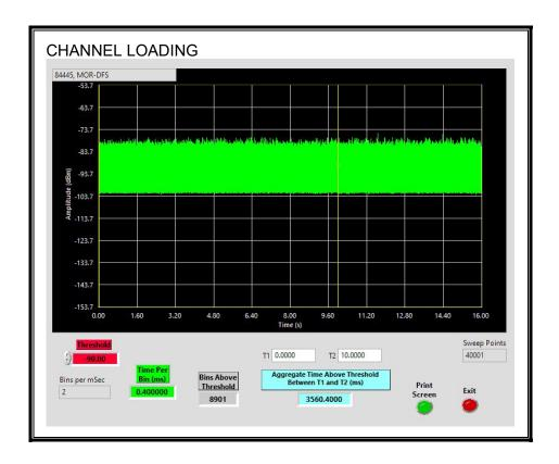
The level of traffic loading on the channel by the EUT is 35.60%
