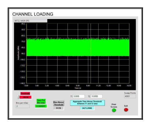
The level of traffic loading on the channel by the EUT is 36.71%
