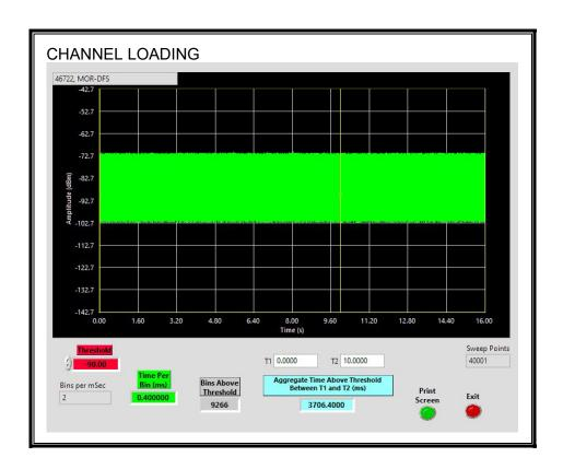
The level of traffic loading on the channel by the EUT is 37.06%
