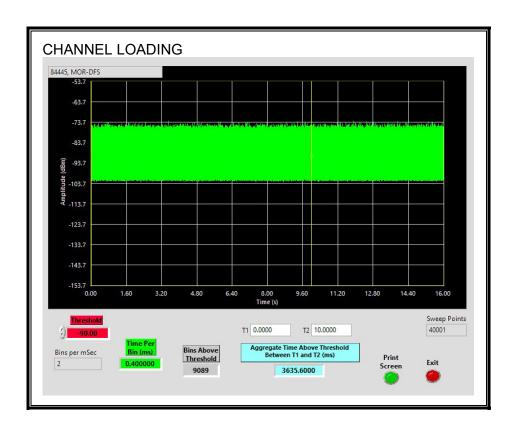
The level of traffic loading on the channel by the EUT is 36.36%
