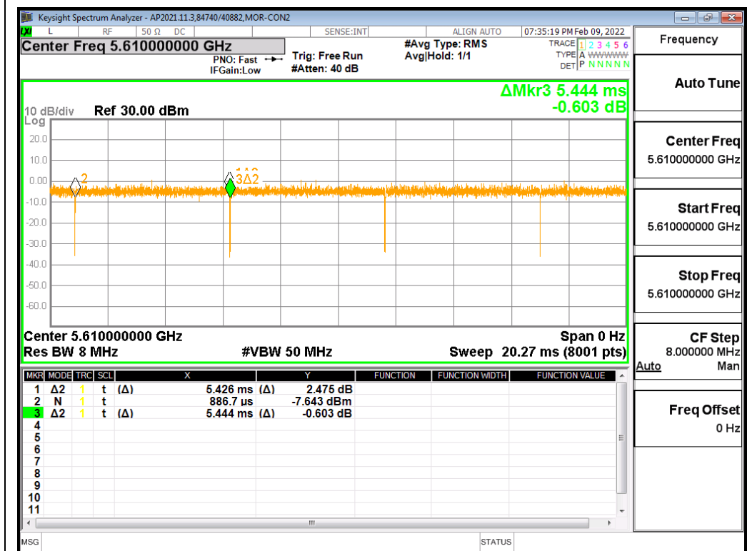
DUTY CYCLE 802.11ac VHT80 MODE
