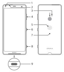
Charging/Notification light 2 Nano SIM/Memory card slot 3 4 Volume/Zoom key 5 Fingerprint sensor 6 Power key 7 Wireless charging coil 8 Camera kev 9 USB port/Charger/Audio adapter
