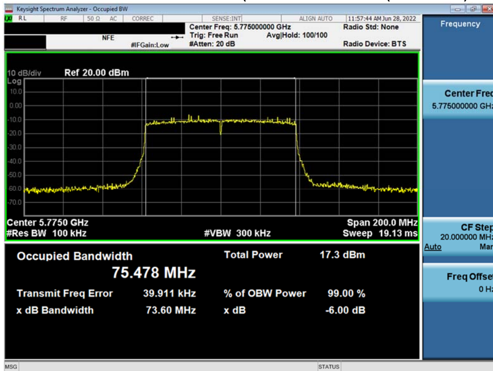
Plot 7-124. 6dB Bandwidth Plot MIMO ANT1 (802.11ac – 80MHz BW (UNII Band 3) – Ch. 155)
