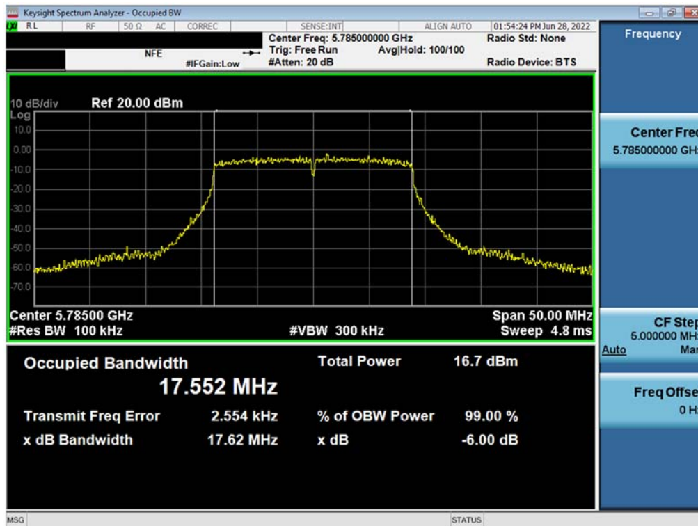
Plot 7-130. 6dB Bandwidth Plot MIMO ANT2 (802.11n – 20MHz BW (UNII Band 3) – Ch. 157)
