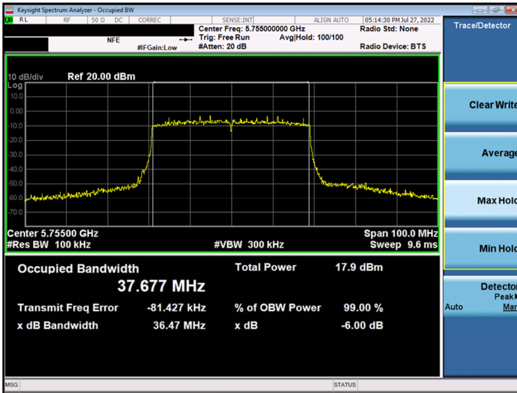
Plot 7-137. 6dB Bandwidth Plot MIMO ANT2 (802.11ax – 40MHz BW (UNII Band 3) – Ch. 151)
