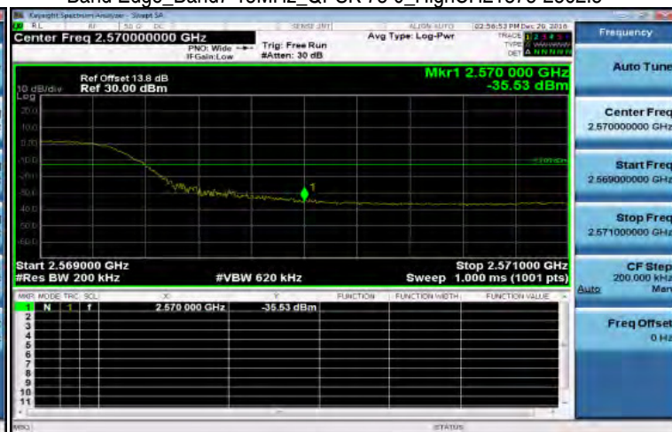
Band Edge_Band7 15MHz_QPSK 75 0_HighCH21375-2562.5
