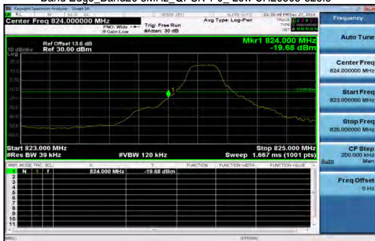
Band Edge_Band26 3MHz_QPSK 1 0_Low CH26805-825.5
