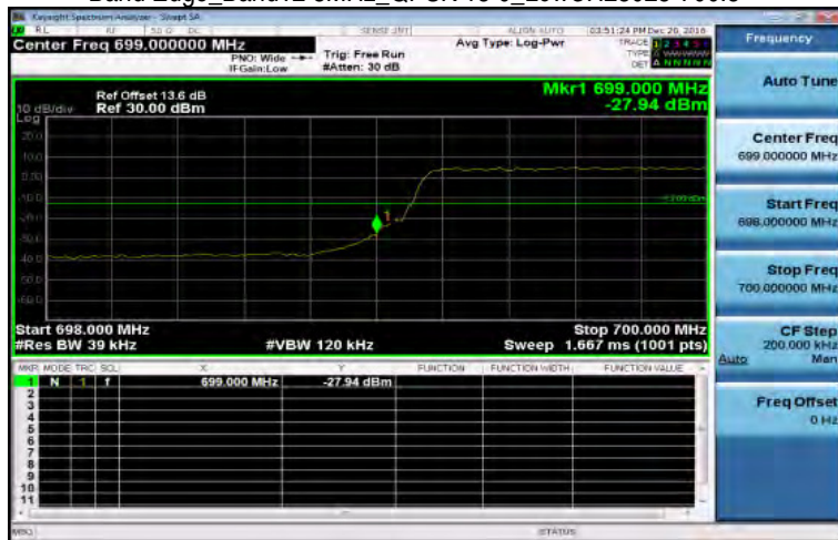
Band Edge_Band12 3MHz_QPSK 15 0_LowCH23025-700.5
