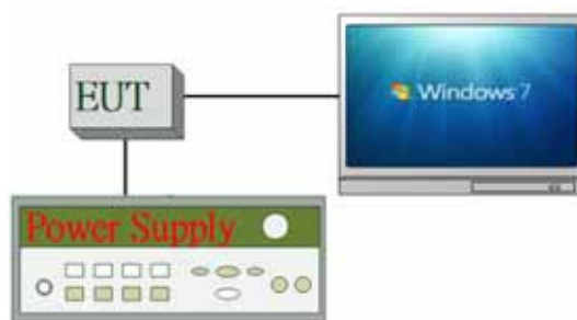
Fig. 2-2 Conducted (Antenna Port) Configuration
