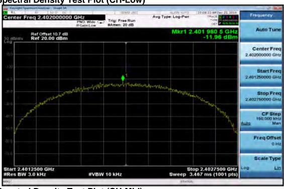
**Power Spectral Density Test Plot (CH-Mid)**
