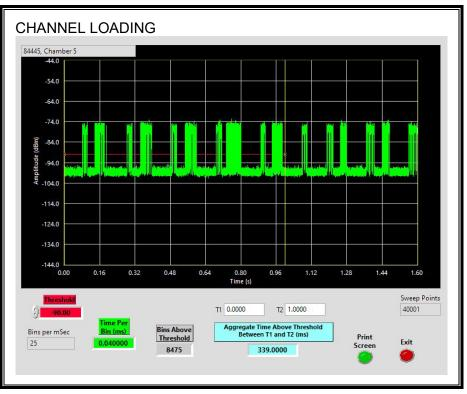
The level of traffic loading on the channel by the EUT is 33.90%
