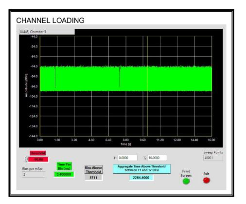
The level of traffic loading on the channel by the EUT is 22.84%
