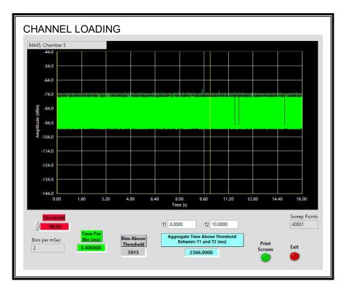
The level of traffic loading on the channel by the EUT is 23.66%
