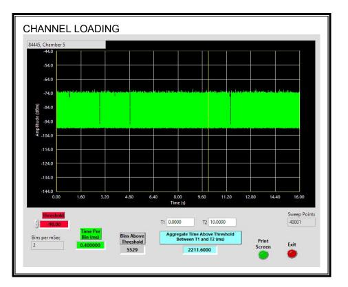
The level of traffic loading on the channel by the EUT is 22.12%
