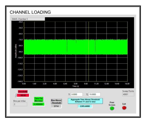
The level of traffic loading on the channel by the EUT is 22.86%
