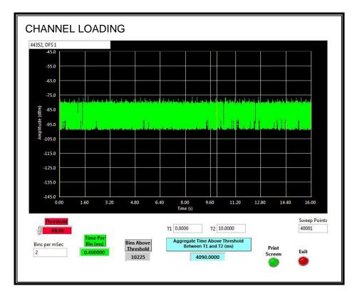
The level of traffic loading on the channel by the EUT is 40.9%.
