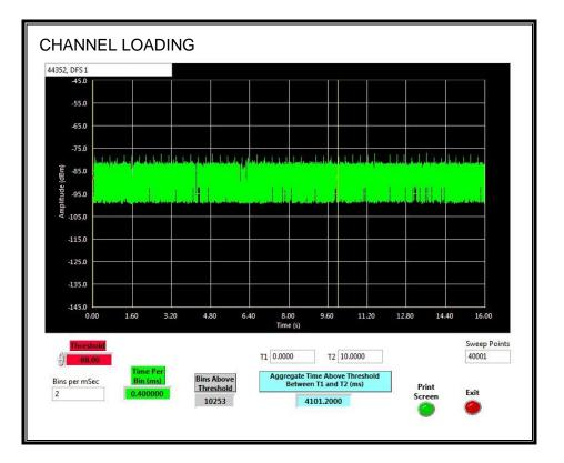
The level of traffic loading on the channel by the EUT is 41.012%.
