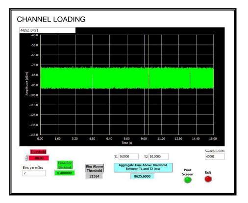
The level of traffic loading on the channel by the EUT is 86.256%.
