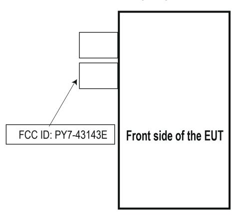
The FCC ID is not on the exterior of the device but labelling meets the conditions allowed in KDB 784748 for the label to be placed in a user accessible area:
