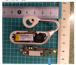
Remove RF shield of the PCB
