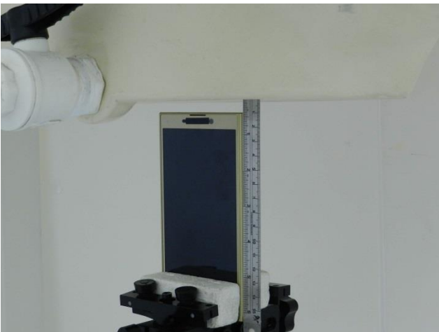
Top Side, Test Separation 10 mm
