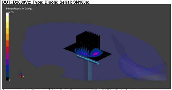
Communication System: CW UID: 0; Frequency: 2600.0 MHz; Duty Cycle: 1; Medium: HSL; Site65\_28Sep2021\_082639\_Head - 900 1800 1900 2300 2600 5%; Medium parameters used: f = 2600.0 MHz;  $\sigma$  = 1.94 S/m;  $\epsilon_r$  = 39.2;  $\rho$  = 1000 kg/m3;  $\Delta \epsilon_r$  = 0.57 %;  $\Delta \sigma$  = 4.02 % No second for the communication  $\epsilon_r$
