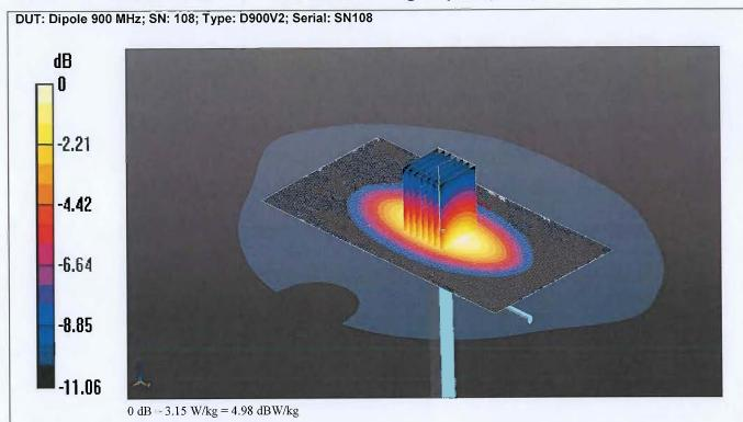
Communication System: UID 0, CW (0); Frequency: 900 MHz; Duty Cycle: 1:1 Medium: 750,835,900,1800,1900 MHz HSL Medium parameters used: f = 900 MHz;  $\sigma$  = 0.967 S/m;  $\epsilon_r$  = 41.565;  $\rho$  = 1000 kg/m³ Phantom section: Flat Section
