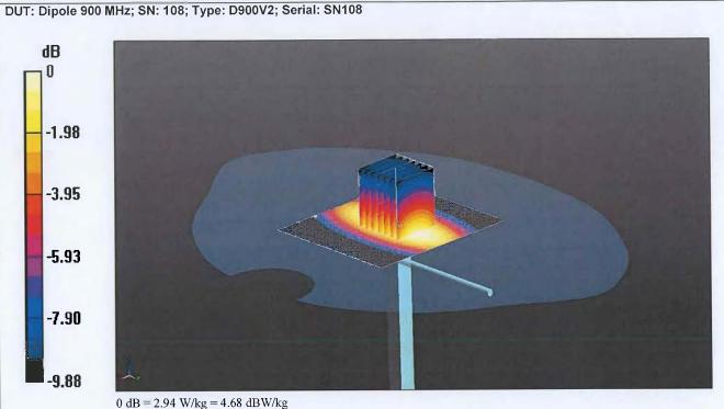
Communication System: UID 0, CW (0); Frequency: 900 MHz; Duty Cycle: 1:1
