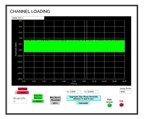
The level of traffic loading on the channel by the EUT is 35.89%.
