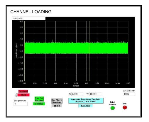
The level of traffic loading on the channel by the EUT is 45.85%.
