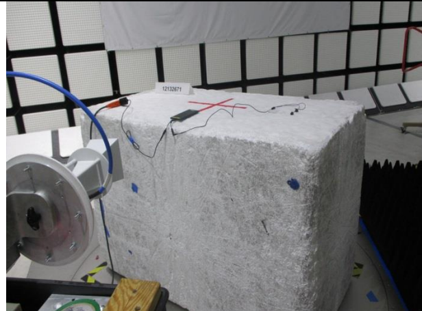
RADIATED FRONT PHOTO (ABOVE 18-40 GHz)
