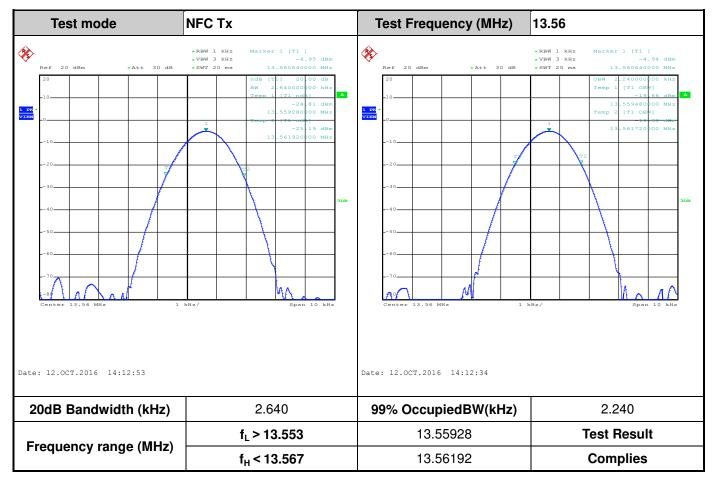
B1. Test Result of 20dB Spectrum Bandwidth
