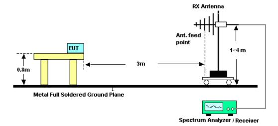
For radiated emissions from 1GHz to 18GHz
