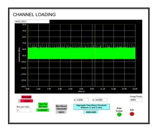
The level of traffic loading on the channel by the EUT is 40.084%.
