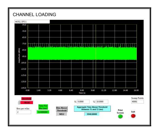
The level of traffic loading on the channel by the EUT is 39.408%.
