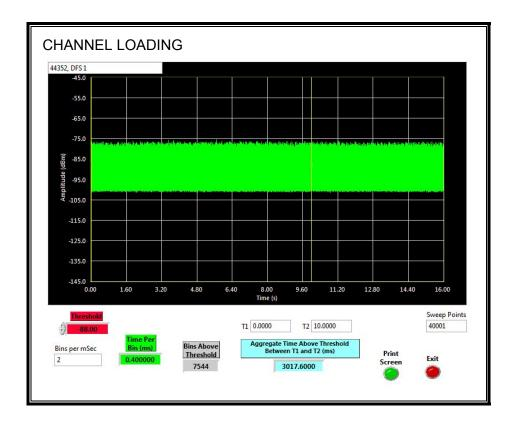
The level of traffic loading on the channel by the EUT is 30.176%.
