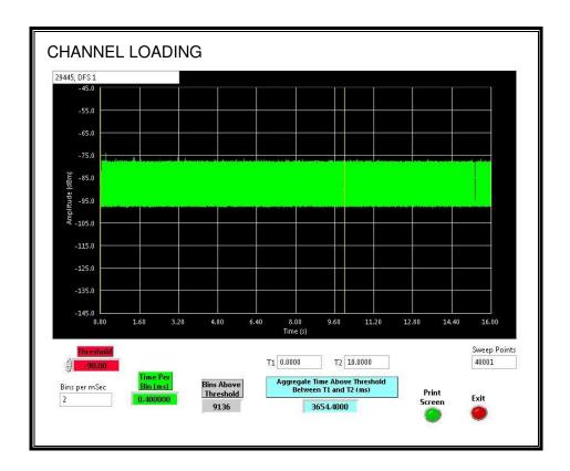
The level of traffic loading on the channel by the EUT is 36.54%
