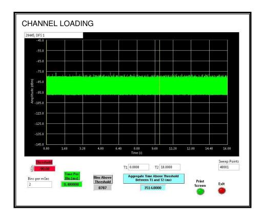
The level of traffic loading on the channel by the EUT is 35.14%
