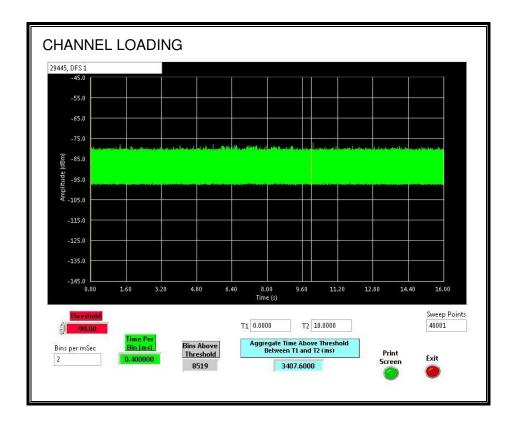
The level of traffic loading on the channel by the EUT is 34.07%
