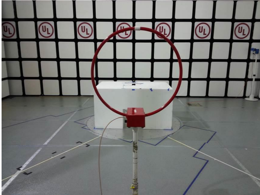
RADIATED EMISSIONS BELOW 30MHz (REAR)
