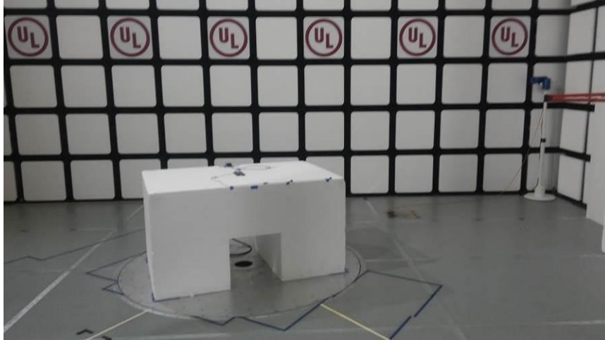
RADIATED EMISSIONS ABOVE 30 MHz (REAR)
