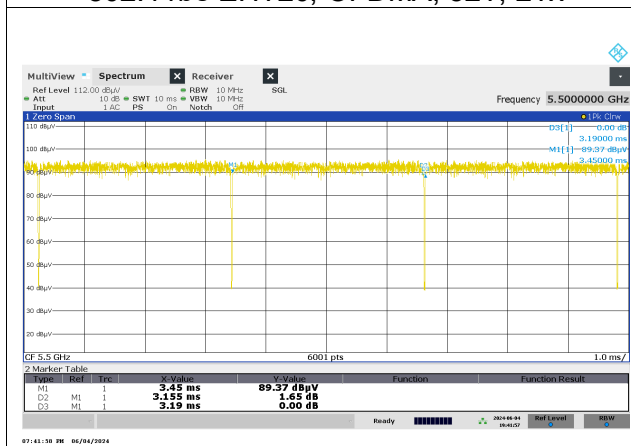
802.11be EHT20, OFDMA, 106T+26T, 2Tx
