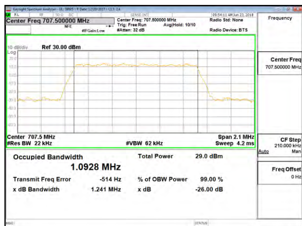
LTE B12 1.4MHz 16QAM Mid Channel RB6-0
