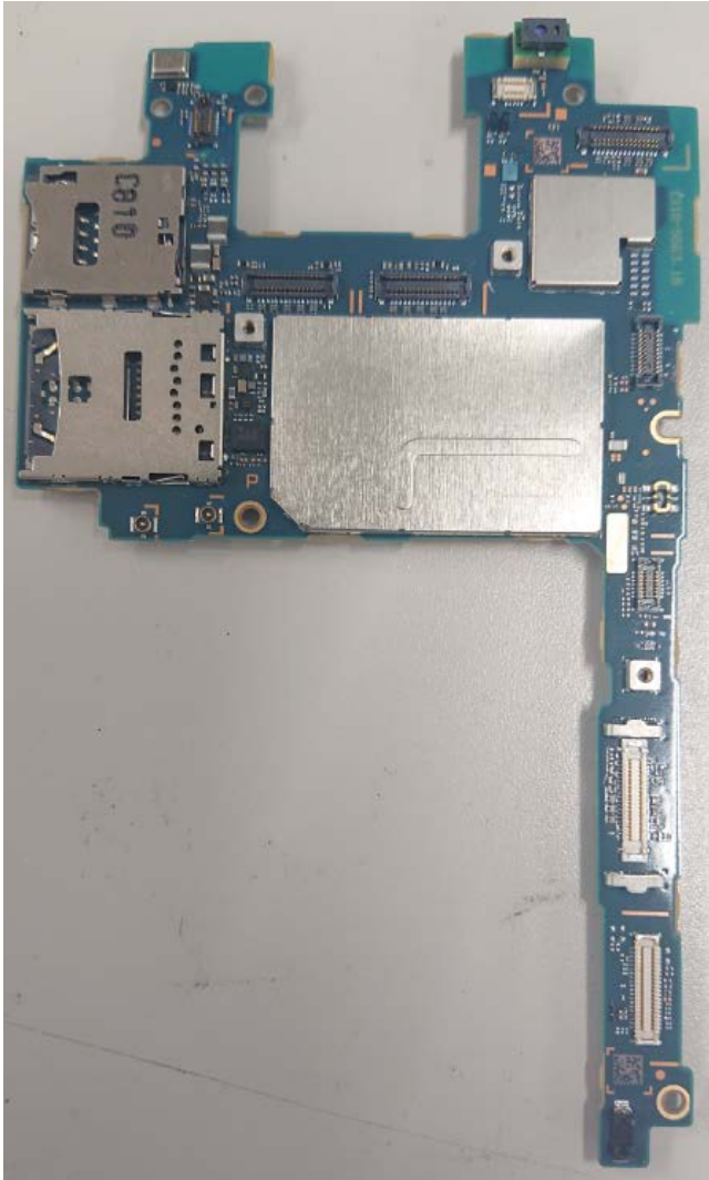
Internal Main PWB with Shield cases (Front-side)
