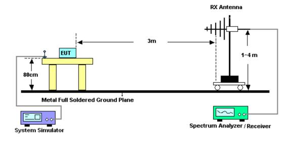
For radiated test from 1GHz to 18GHz
