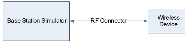
Figure 9-3 Power Measurement Setup
