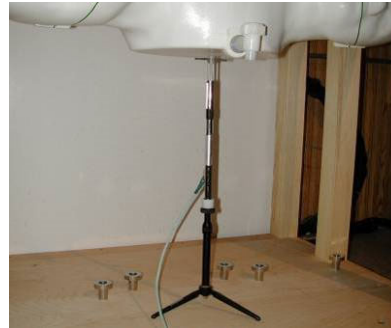
Figure 10-2 System Verification Setup Photo
