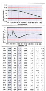
Figure D-3 600 – 10000 MHz Head Tissue Equivalent Matter
