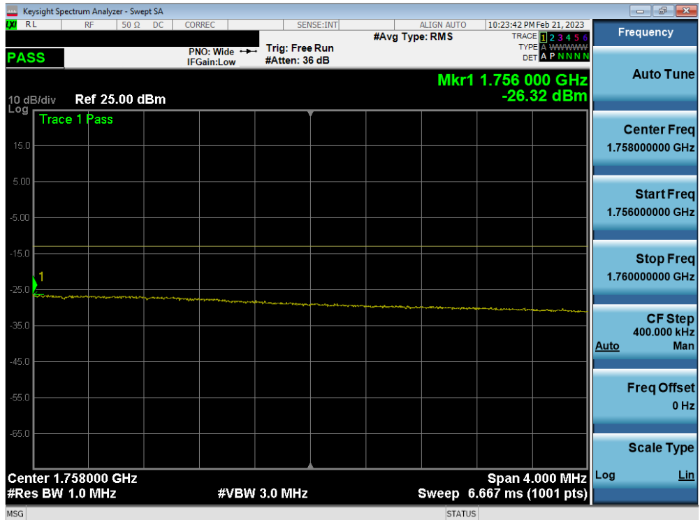
Plot 7-99. Upper Extended Band Edge Plot (LTE Band 4 - 15MHz QPSK – Full RB)
