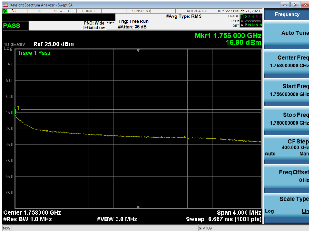
Plot 7-111. Upper Extended Band Edge Plot (LTE Band 4 - 5MHz QPSK – Full RB)
