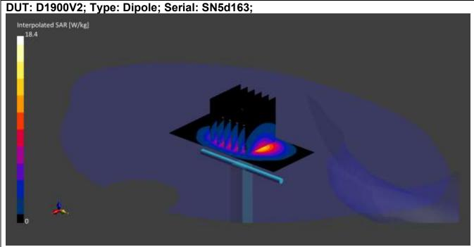
Communication System: CW UID: 0; Frequency: 1900.0 MHz; Duty Cycle: 1; Medium: HSL; Site65\_28Sep2021\_082639\_Head - 900 1800 1900 2300 2600 5%; Medium parameters used: f = 1900.0 MHz;  $\sigma$  = 1.44 S/m;  $\epsilon_r$  = 40.3;  $\rho$  = 1000 kg/m3;  $\Delta\epsilon_r$  = 0.66 %;  $\Delta\sigma$  = 2.96 %; No correction
