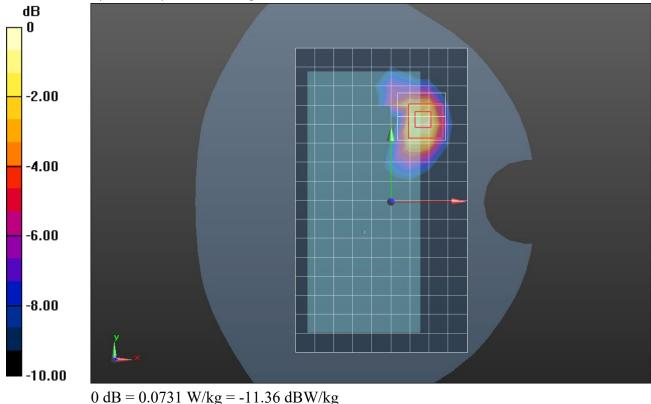
Frequency: 2462 MHz; Duty Cycle: 1:1; Room Ambient Temperature: 24.0°C; Liquid Temperature: 23.0°C Medium parameters used (interpolated): f = 2462 MHz;  $\sigma$  = 1.806 S/m;  $\epsilon_r$  = 37.405;  $\rho$  = 1000 kg/m<sup>3</sup> DASY5 Configuration:
