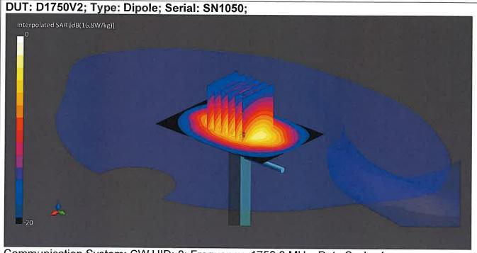
Communication System: CW UID: 0; Frequency: 1750.0 MHz; Duty Cycle: 1; Medium: HSL; Site65\_12Apr2021\_115940\_Head - 1750 1800 1900 2300 2450 2600 5%;
