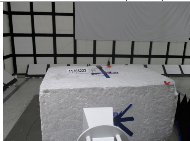
RADIATED FRONT PHOTO (18-40 GHz)
