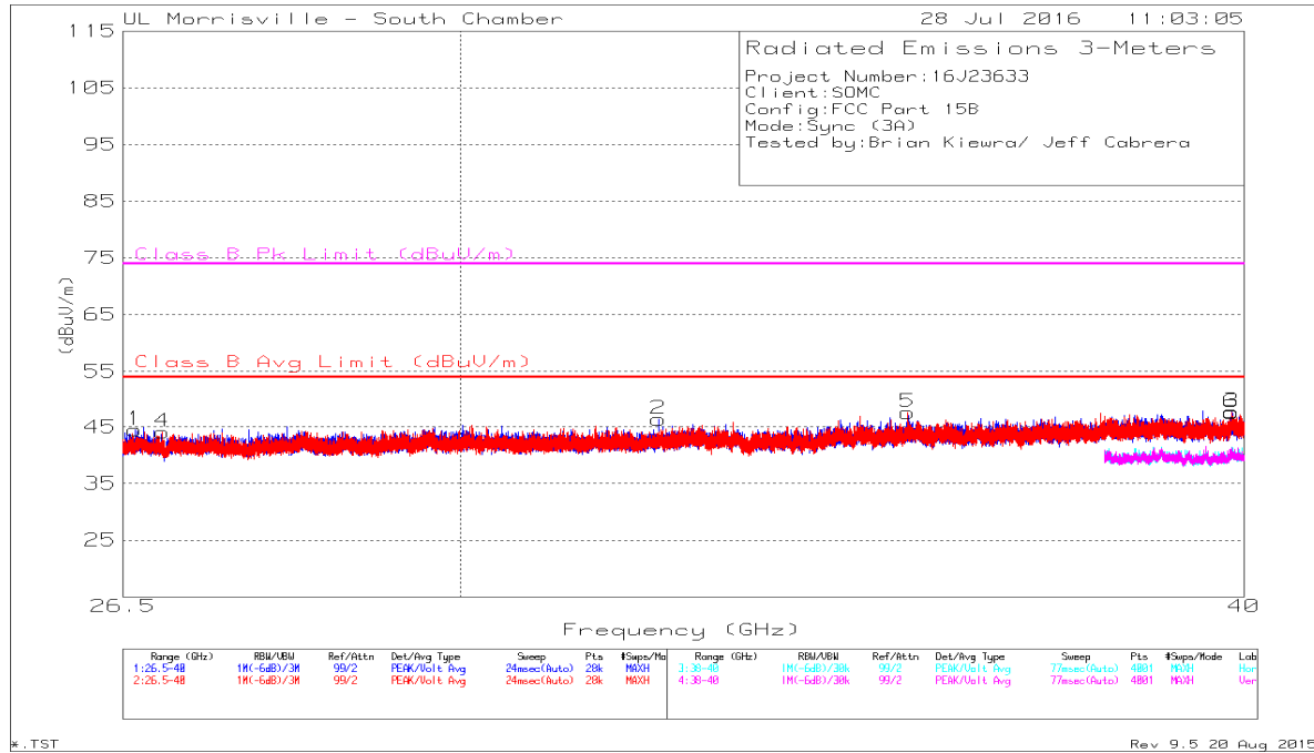
Figure 18 Radiated Emissions Graph – 26-40 GHz Sync
