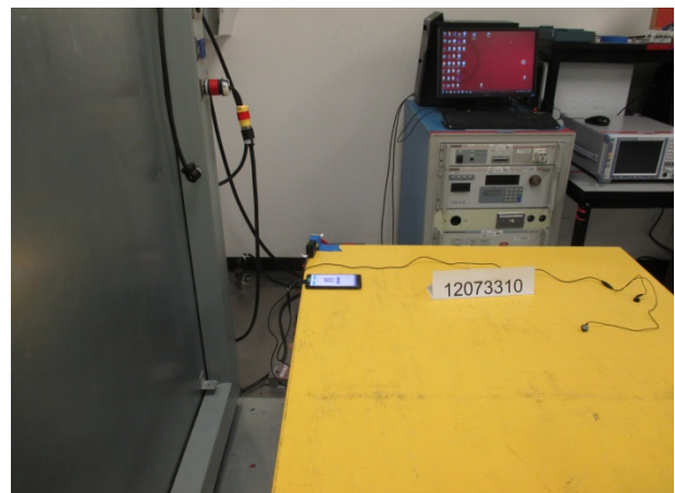
LINE CONDUCTED FRONT PHOTO (CHARGING MODE)
