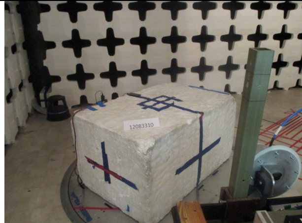
RADIATED FRONT PHOTO (ABOVE 18-40 GHz)
